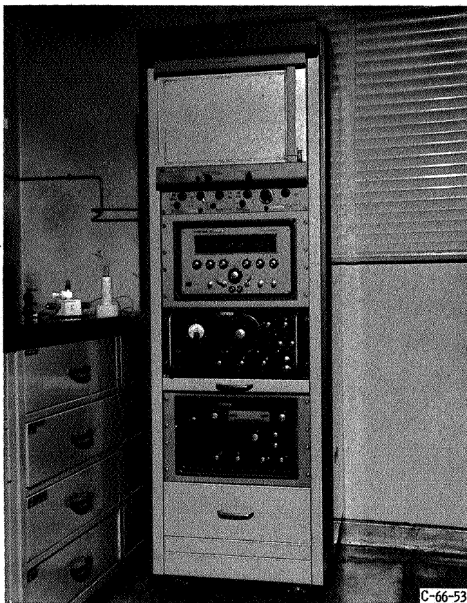
Figure 4. - Bridge and associated equipment used for capacitance measurements.
