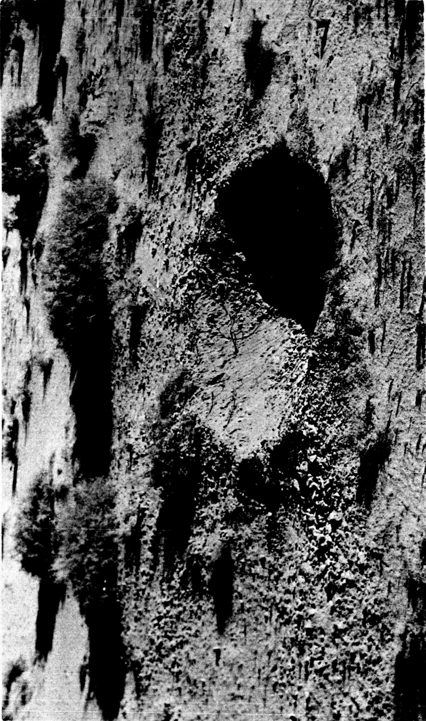
Figure 5.--Missile impact in layered material. Upper layer is very weakly cohesive sand and silty sand. Lower layer is weakly cohesive silt and sand with uniform structure. Crater is about 6 m across. (Oblique aerial photograph courtesy of U.S. Army).
