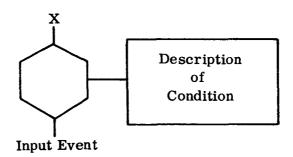
RANDOM INHIBIT Gate. The RANDOM INHIBIT Gate is functionally the same as the INHIBIT Gate. However, in this case the conditional input is a variable.
