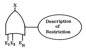
Other Symbols. In addition to the gates, several other symbols are used in the construction of fault trees.
