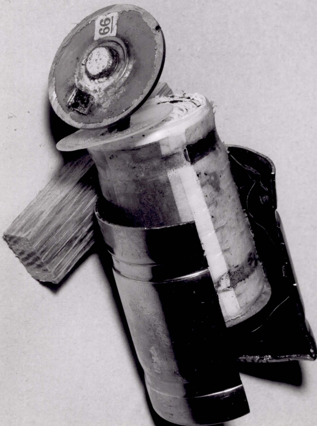
Cell No. 66 Sonotone, 19906 Cycles 10% Depth at 25°C
