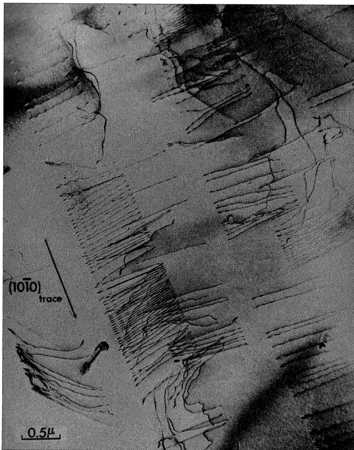
FIG. 18 Dislocation arrangements after \sim 3\% deformation (b) Coplanar arrays in quenched Ti:8.65 wt% Al
