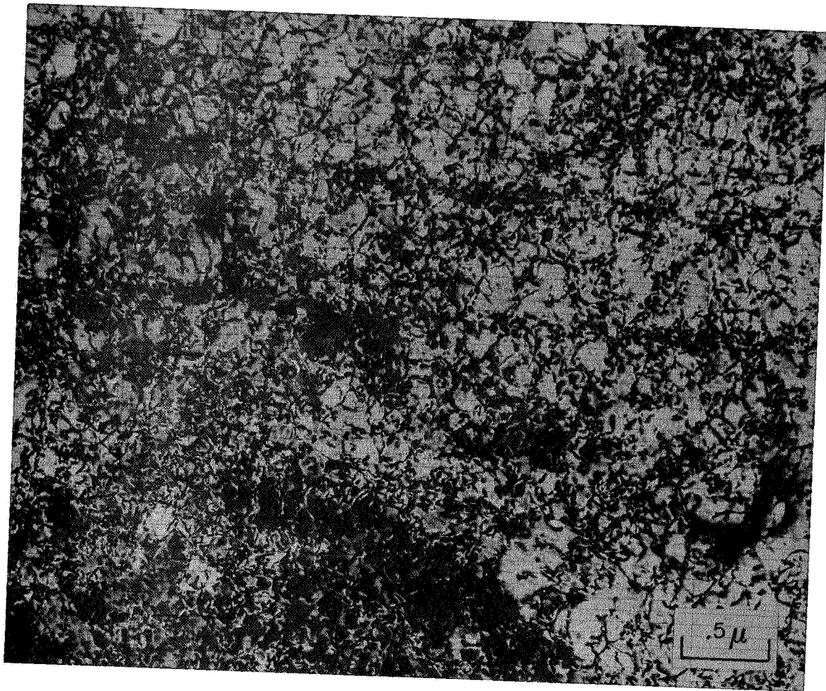
FIG. 18 Dislocation arrangements after ~3% deformation (a) Extensive tangling in commercially pure titanium ( 1500 ppm oxygen)
