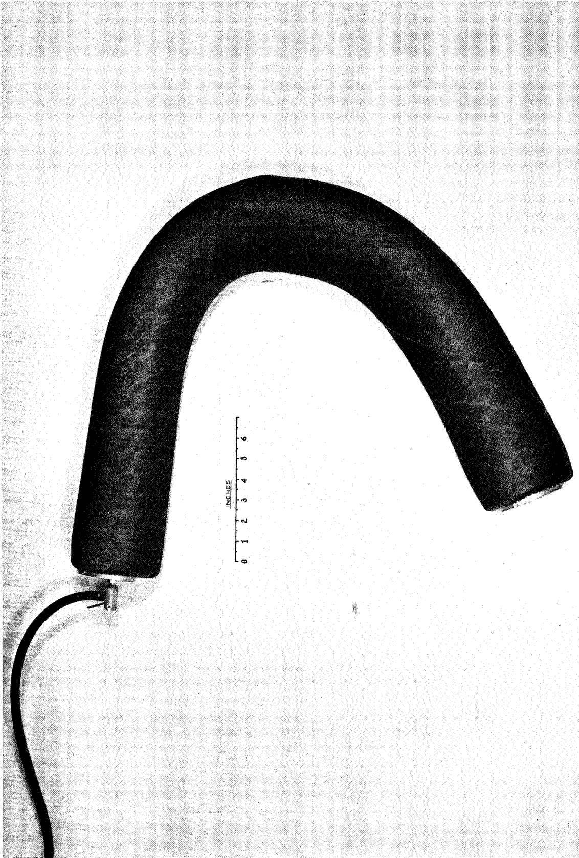
FIGURE 9. PRESSURIZED THREE-LAYER SLIP-NET TUBE MADE FROM "TEFLON" - BENT
