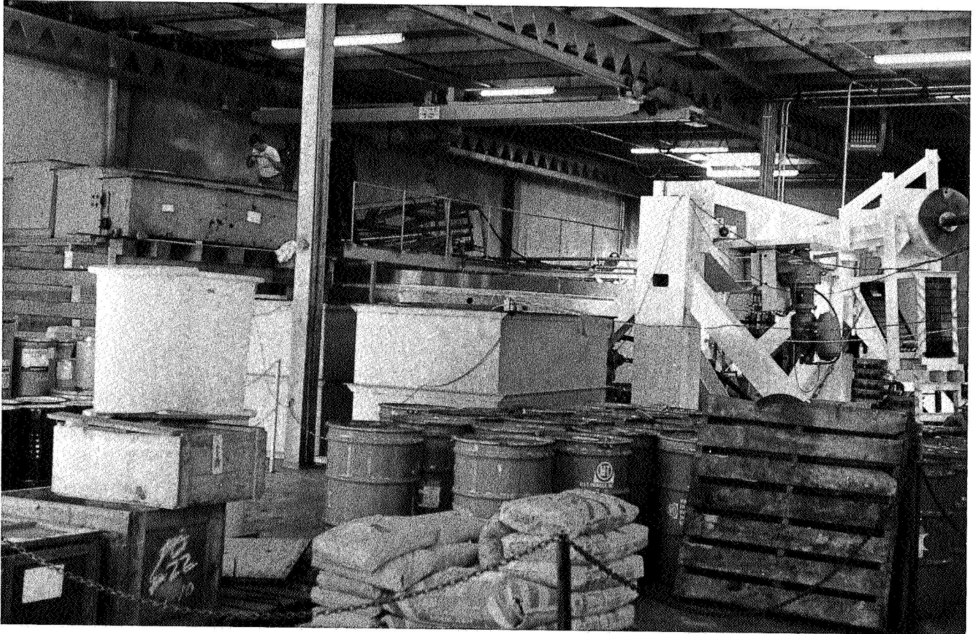
Fig. 5. Tanks containing cleaning, etching, and plating solutions
