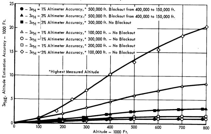
first measurement was made is equally dependent on highest altitude of operation and greatest altimeter accuracy. Figure 4.6-2 shows that the density estimation error is more dependent on altimeter accuracy. A maximum altitude of 200,000 feet and an altimeter accuracy of 1% (3  $_{\rm J}$ ) was selected as the combination to best fulfill the entry science data requirements.
