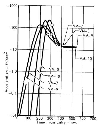
$V_{e} = 15,000 \text{ ft/sec}$   $y_{e} = -14.1 \text{ deg}$
