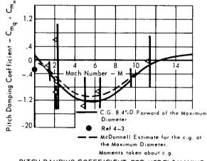
EFFECT OF MACH NUMBER ON PITCHING MOMENT COEFFICIENT SLOPE
