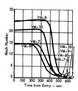
$V_e = 15,000 \text{ ft/sec}$  $\gamma_e = -14.1 \text{ deg}$
