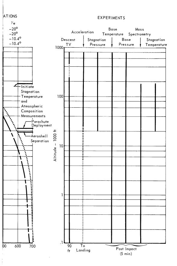
High speeds may affect the operating temperatures of some sensors. Consequently, the stagnation temperature measurements and mass spectrometer sampling are not initiated until the capsule decelerates to about Mach 5. The peak dynamic pressure is used as a reference point for timing the start of these measurements. After the parachute deployment and Aeroshell separation, terminal propulsion rocket plumes will affect the measurements of the stagnation temperature and pressure sensors.
