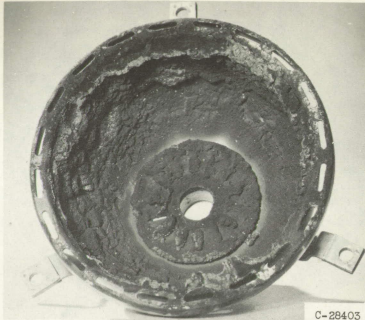
(c) On dome and primary-air entry ports after 30-hour run with JP-3 fuel.
