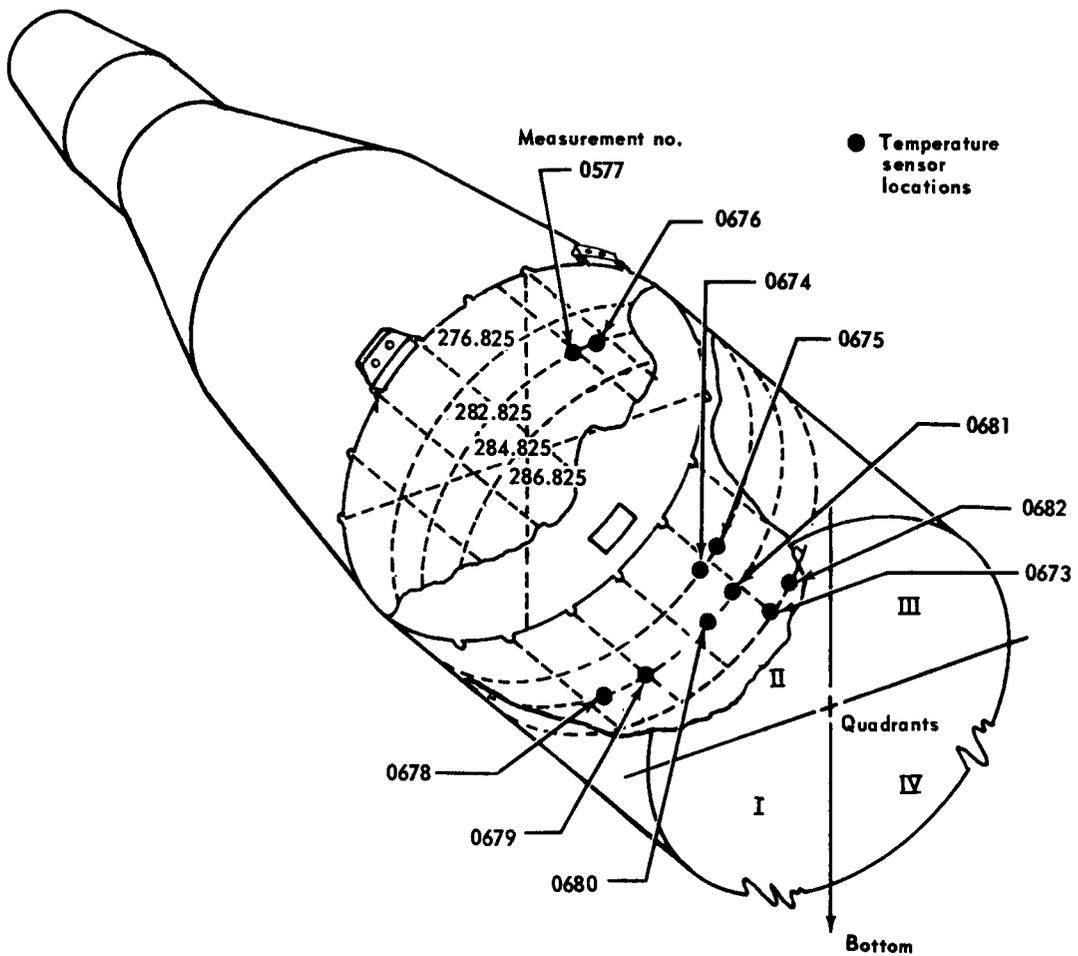
FIGURE 5-21 INTERFACE THERMOCOUPLE LOCATIONS
