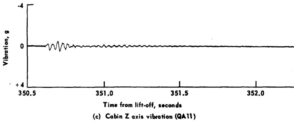
FIGURE 5-35 SPACECRAFT VIBRATION MEASUREMENTS AT LIFT-OFF +351 SECONDS
