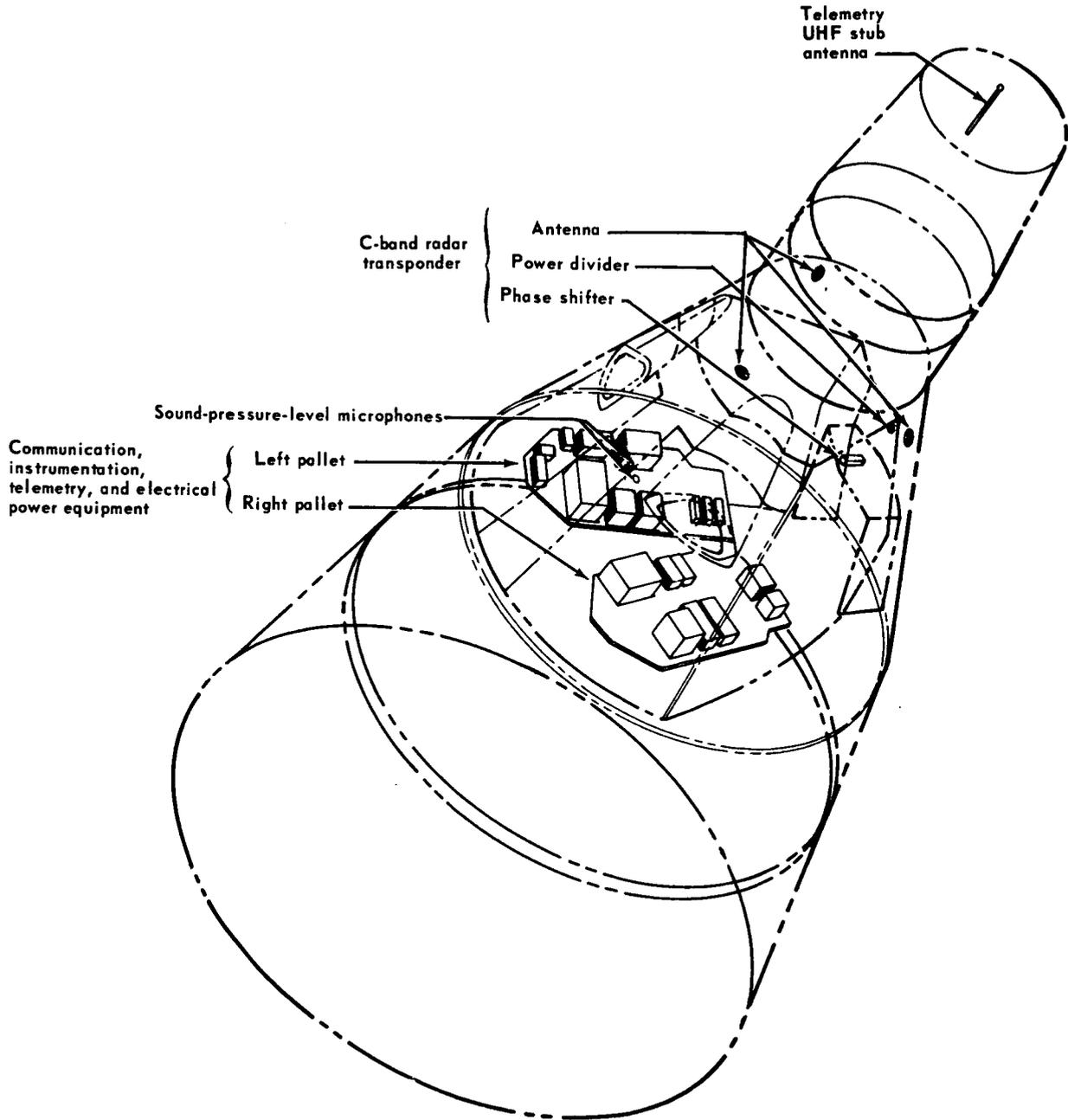
FIGURE 3-4 INSTRUMENTATION, COMMUNICATION, TELEMETRY, AND ELECTRICAL SYSTEM EQUIPMENT LOCATION ON SPACECRAFT
