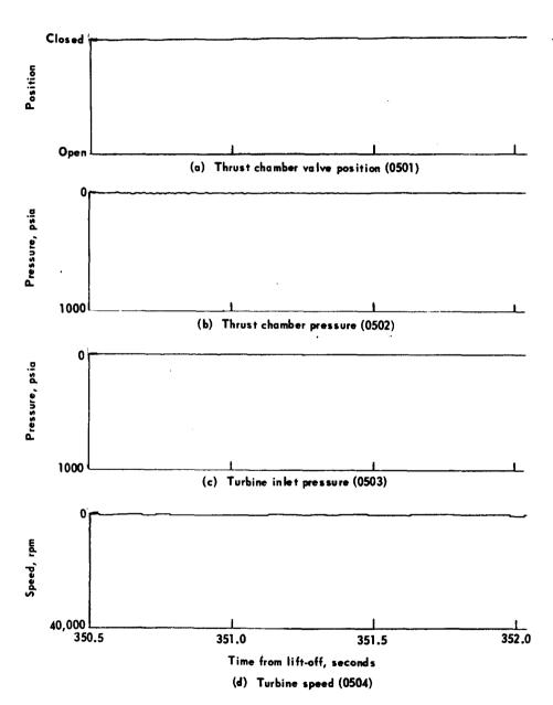
FIGURE 5-34 GLV STAGE II MEASUREMENTS AT LIFT-OFF +351 SECONDS
