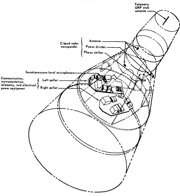
FIGURE 3-4 INSTRUMENTATION, COMMUNICATION, TELEMETRY, AND ELECTRICAL SYSTEM EQUIPMENT LOCATION ON SPACECRAFT
