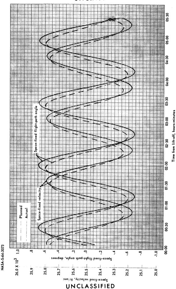
(b) Space-fixed velocity and flight-path angle.
