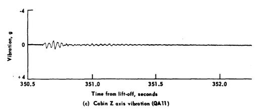
FIGURE 5-35 SPACECRAFT VIBRATION MEASUREMENTS AT LIFT-OFF +351 SECONDS
