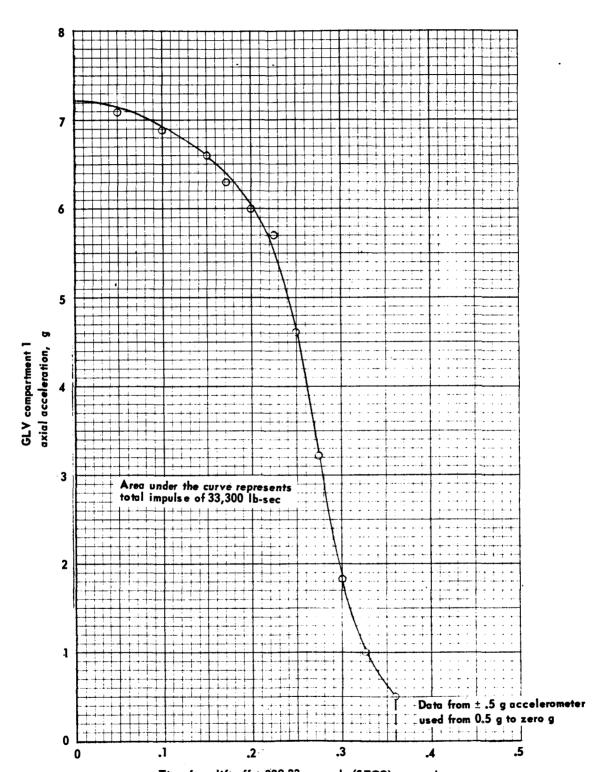
Time from lift-off + 339.23 seconds (SECO), seconds (a)  $\pm 10g$  accelerometer
