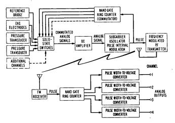
transmitter part of the system. The lower part of the figure is the receiving and demodulating equipment that provides an analog signal suitable as an input to a pen recorder.
