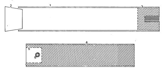
A technique has been developed, for X-raying welded and brazed tubing joints, which produces a clear continuous picture of each joint on a single film with one exposure. Conventional techniques require multiple films and exposures to obtain a clear and complete picture of a single joint.
