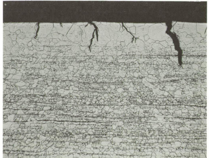
Fig. B-5. Section of reservoir base plate showing surface cracks resulting from post-test removal of lithium by water (100 X) (Photo reduced to 75%)
