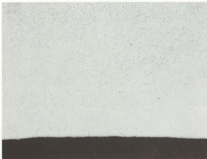
Fig. B-2. Inner diameter of niobium alloy piping after 500 hr at 1073–1143°C (Photo reduced to 75%)
