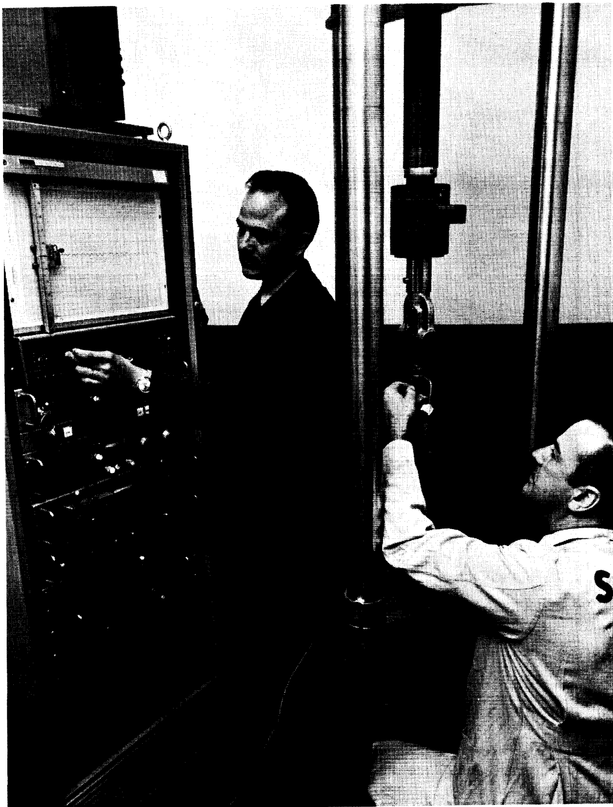
FIGURE 5. MTS AXIAL FATIGUE CLOSED LOOP TESTING MACHINE
