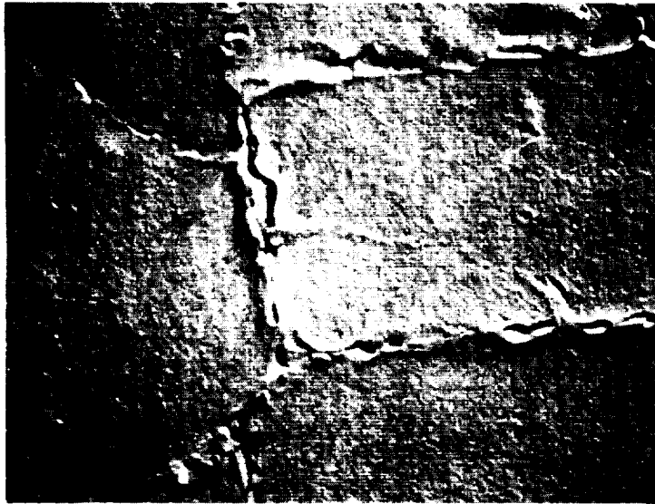
Material: 0.209-inch Inconel 718 alloy Note absence of denuded zone along grain boundaries. Magnification: 15,000X
