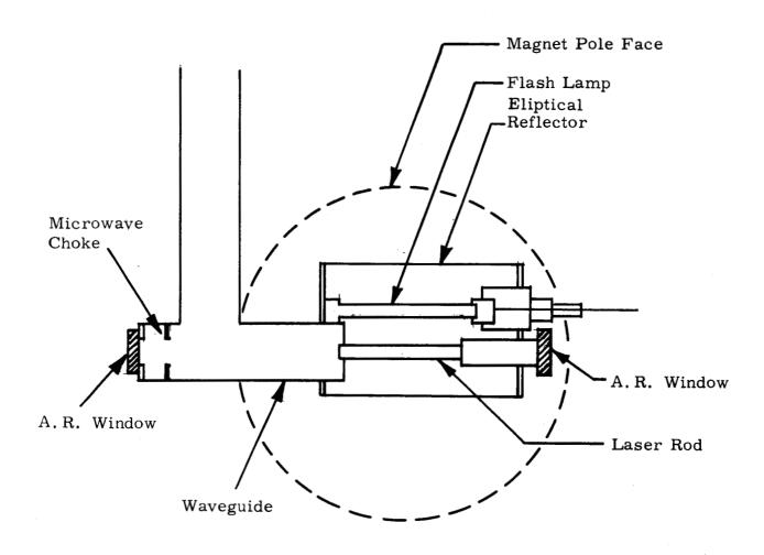
Fig. 4. Schematic diagram of sample mounting in magnet pole gap.
