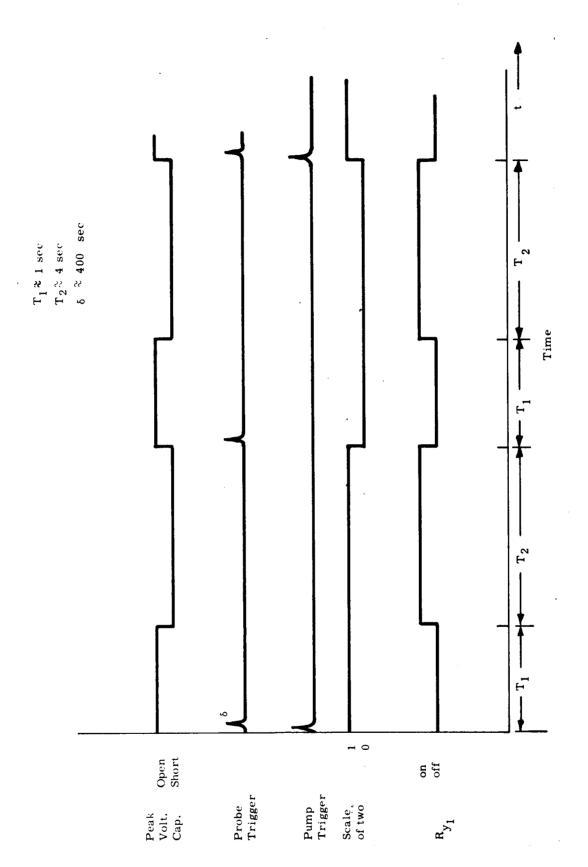
Fig. 7. Timing sequence diagram.
