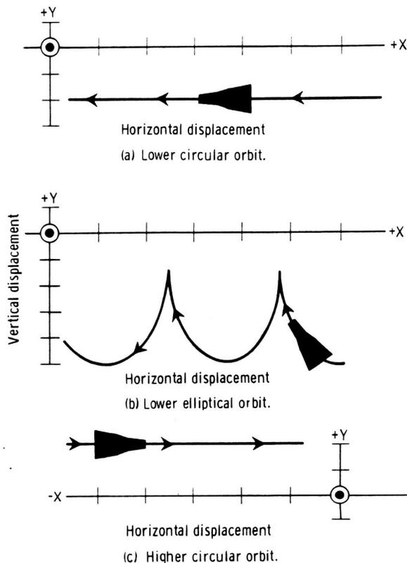
FIGURE 2-2.—Motion relative to a target-centered coordinate system.
