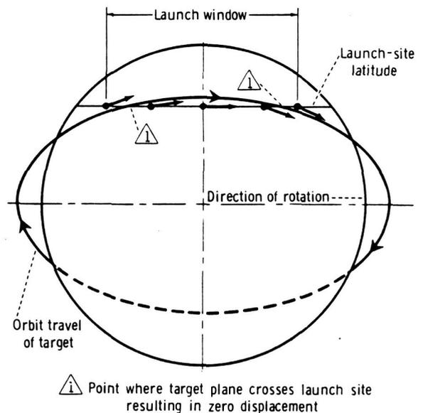
FIGURE 2-13.—Variable azimuth launch technique.
