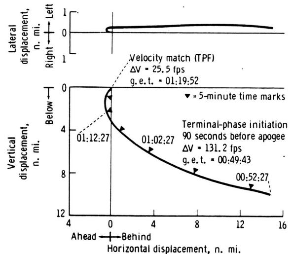
FIGURE 2-8.—Relative trajectory, terminal phase. Gemini XI mission.
