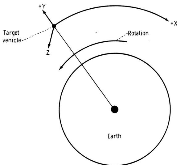
FIGURE 2-1.—Target-centered coordinate system.
