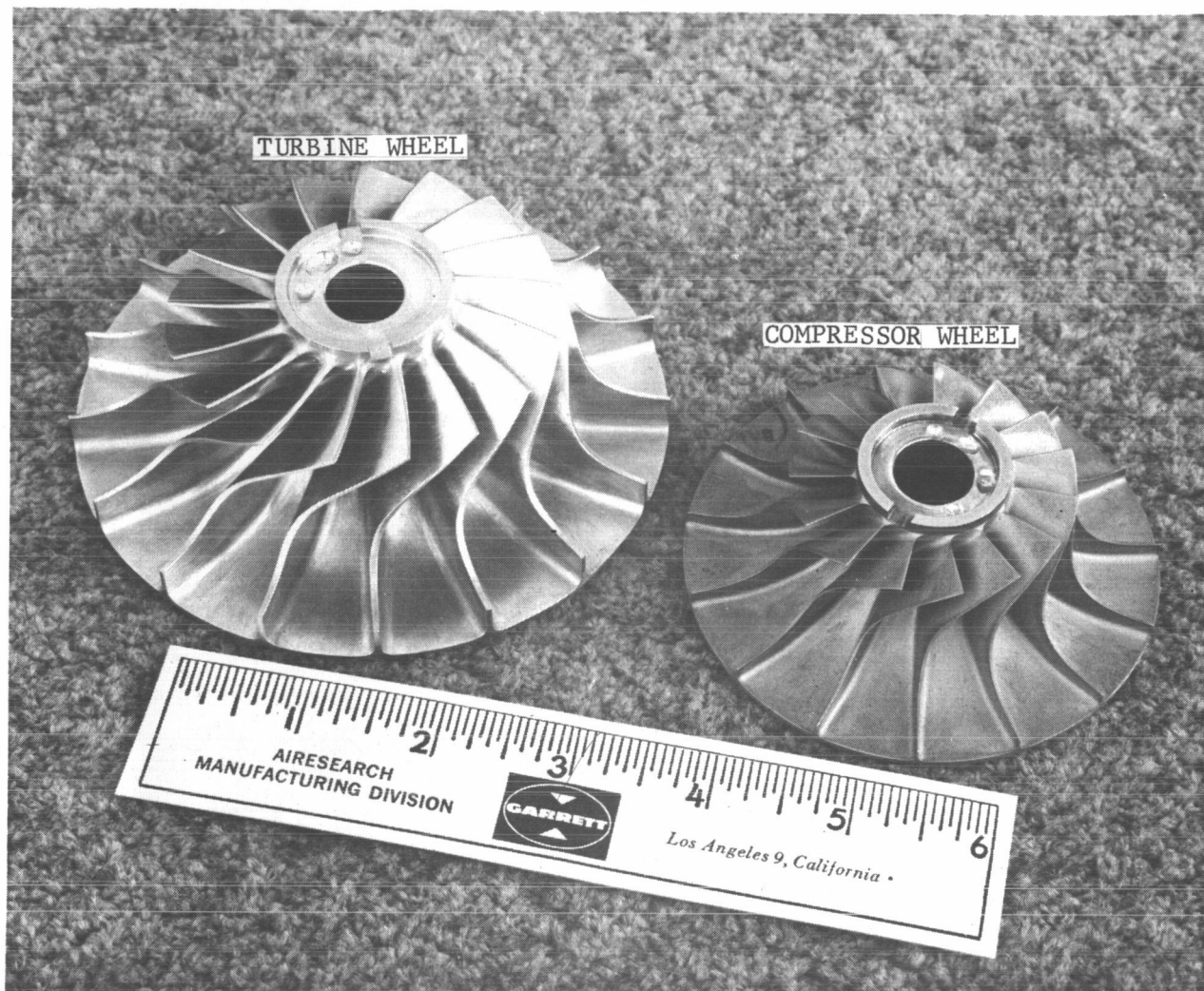
FIGURE 10 BCD COMPRESSOR AND TURBINE WHEELS
