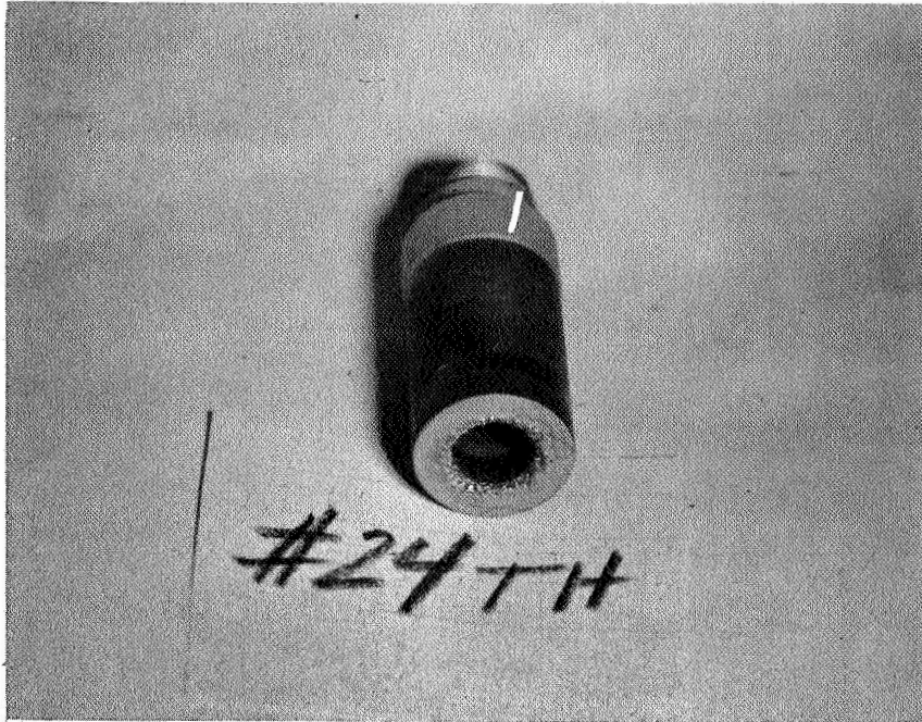
Figure 33: Photograph of Hollow Cathode After Testing, 500 A, 3.5 psig
