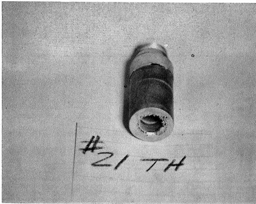
Figure 34: Photograph of Hollow Cathode After Testing, 500A, 15 psig
