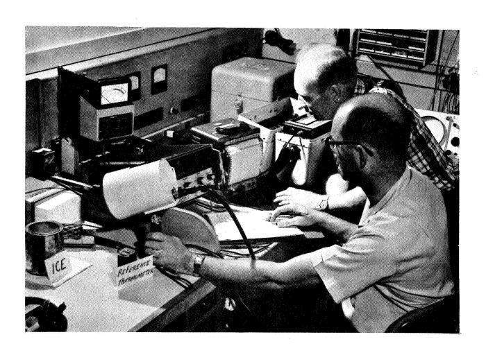
Figure 5.--Ross substation instrument laboratory personnel check accuracy of PRT-5 radiometer and correlate Varian recorder readings with PRT-5 radiometer output.
