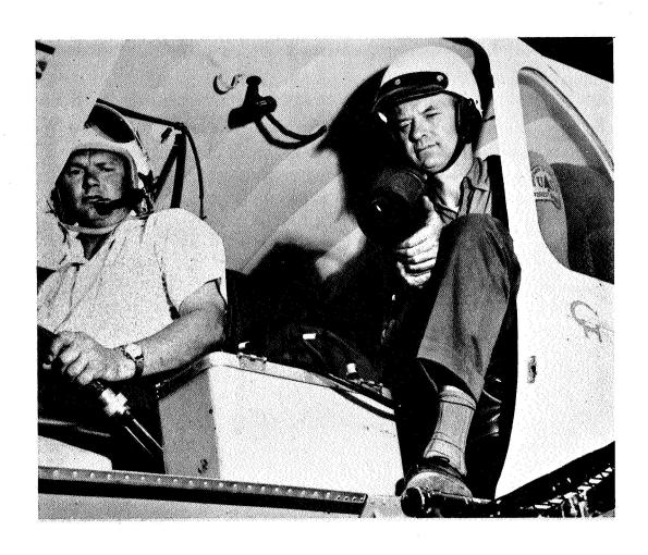
Figure 4.--Operator using a Barnes PRT-5 radiometer to record infrared heat emissions from individual trees. The helicopter is flown about 150 feet above the trees in a flat circling pattern around each specifically marked tree.
