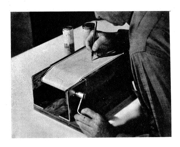
Figure 6.==Data from the Varian recorder chart rolls are easily tabulated when using this simple roller device. The temperature indications at systematic intervals are collected, averaged, and converted into a Fahrenheit temperature for each tree.
