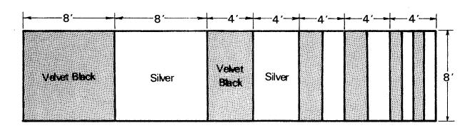
Four feet by eight of Celotex fibre board covered with paper-backed foil and alternately painted with 3M velvet black paint.
