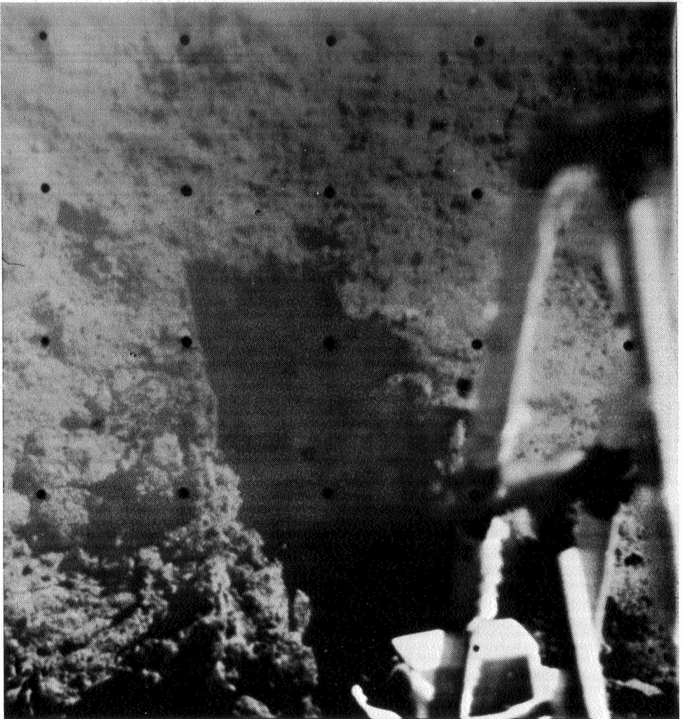
Fig. 31. Narrow-angle view of surface sampler having completed a second pass digging a trench. Object near the top was thought to be a rock; later events determined that it was not
