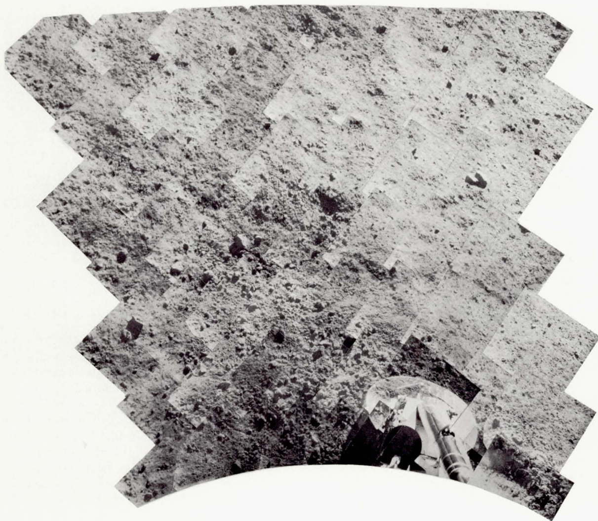
FIGURE 4-8. — Narrow-angle mosaic of footpad 2 and some of the lunar material ejected during the landing and the formation of the trench (day 255, about 10:11 GMT; catalog 5-MP-26).
