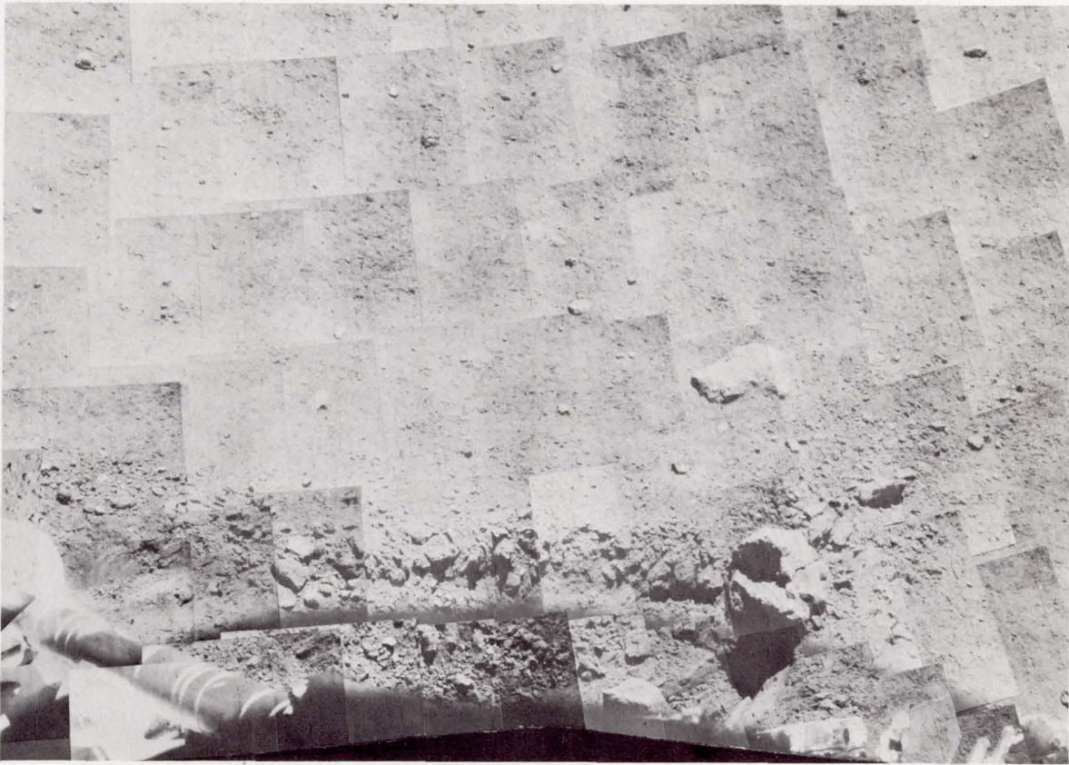
FIGURE 4-7. — Narrow-angle mosaic showing the trench formed by footpad 2 during the spacecraft landing (day 258, about 08:00 GMT; catalog 5-MP-34).
