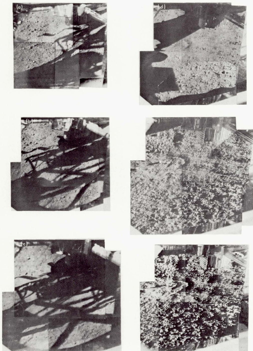
FIGURE 4-22. — A series of narrow-angle mosaics of the lunar surface beneath vernier engine 3. The series includes two prefiring (a and b) and four postfiring pictures. Sun elevation relative to the local surface was 33°, 44°, 40°, 31°, 20°, and 16° (a to f, respectively). Two spacecraft tanks and the electronics box on the left bound the pictures. A spacecraft structural member divides the visible lunar surface.
