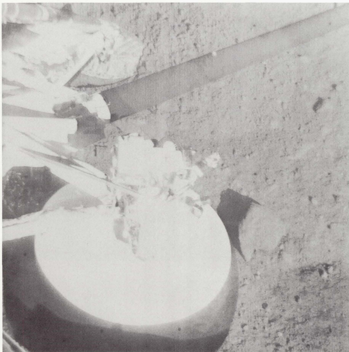
FIGURE 4-12. — Wide-angle picture of footpad 3. The footpad imprint in the lunar material can be seen above the antenna boom. The footpad remained tilted after the landing phase. Ghost image of the helium tank was caused by incomplete erasure of previous image on vidicon (day 254, 23:50:28 GMT).
