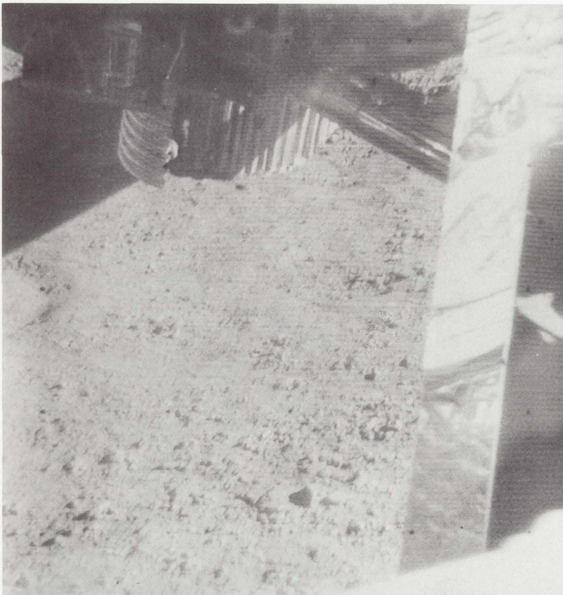
FIGURE 4-14. — Narrow-angle view taken through the auxiliary mirrors showing the bottom of crushable block 3. A small rock or clod, seen wedged between the block and the thermal shield, was probably picked up during the first landing impact (day 263, 11:47:23 GMT).
