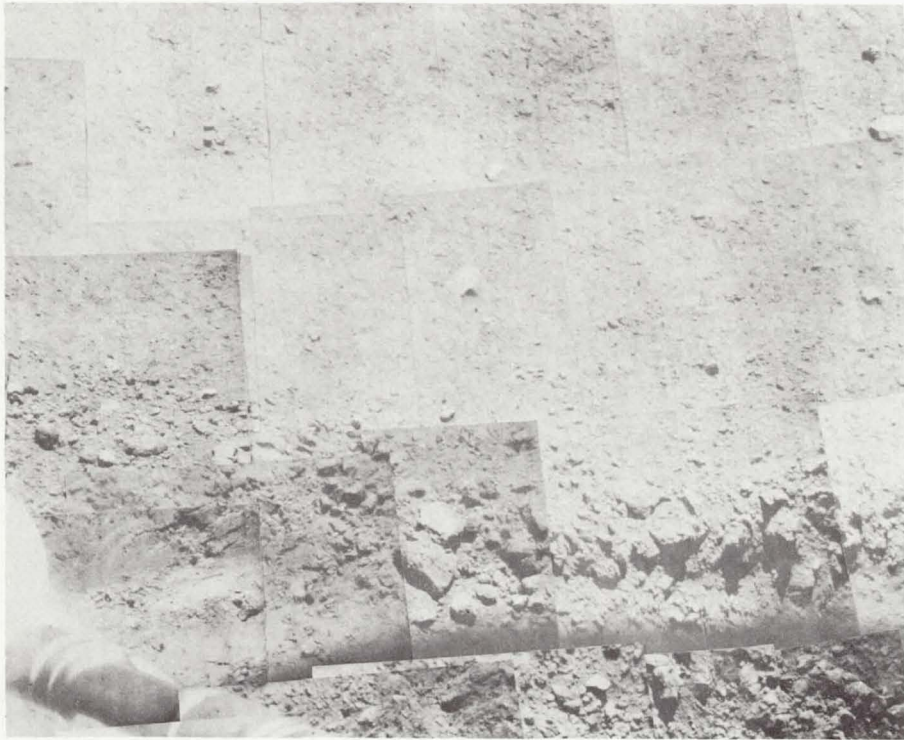
FIGURE 4-38. — Postfiring mosaic of the same portion of footpad 2 trench seen in the prefiring mosaic (fig. 4-37). No disturbance was caused by the firing of vernier engine 2, which was approximately 1 meter away (day 258).
