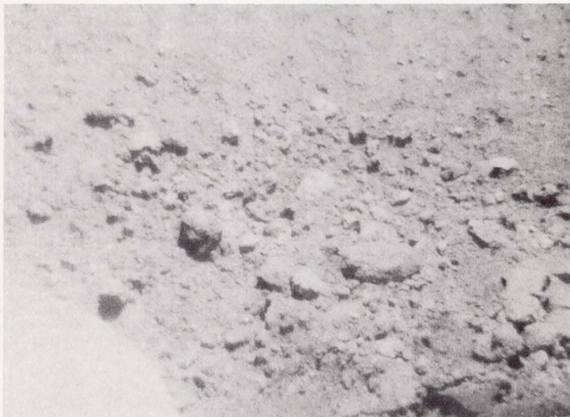
FIGURE 3-18. — Area V-A, used to determine size-frequency distribution of fragmental material thrown onto the lunar surface in front of footpad 2 during landing. Most of the fragments are aggregates of fine particles. The bright fragments probably are pieces of coherent rock. Some dark, lumpy objects may be aggregates of aggregates. Smallest fragments resolved in this picture are about 1 mm across, and the largest fragments are about 3 cm across (day 258, 08:40:04 GMT).
