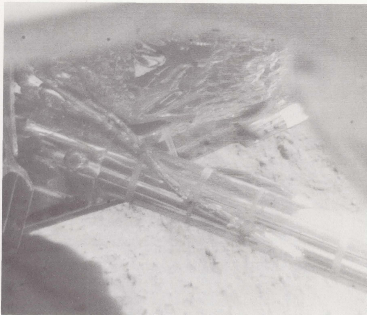
FIGURE 4-24. — A postfiring view of the only part of the vernier engine 1 impact area that can be seen by the television camera. The rough-textured lunar surface within the small triangular area is probably part of an erosion crater. This area was in shadow before the firing (day 263, 11:47:05 GMT).
