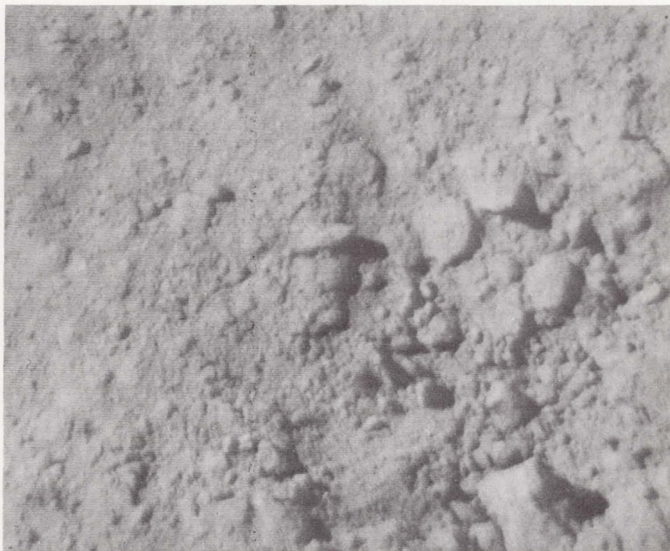
FIGURE 3-20. — Narrow-angle picture showing fragments in small crater on the north wall of the Surveyor V crater. The small crater is lined with fragments similar to those exposed in the trench dug by footpad 2 during landing. Most of the fragments are aggregates of fine particles; complex aggregates and individual bright rocky chips also appear to be present (day 264, 12:12:24 GMT).
