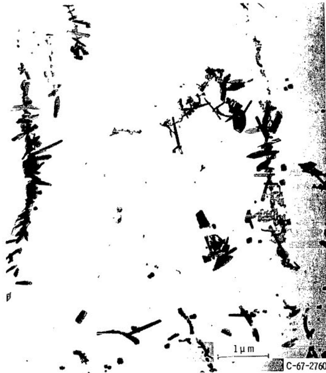
Figure 21. - Electron micrograph of extraction replica of cast alloy \text{Co} - \frac{7}{2}\text{W} - \frac{2}{2}\text{Fe} - 1\text{Ti} - \frac{1}{2}\text{Zr} - \frac{1}{2}\text{C} aged 72 hours at 1700^\circ\text{F} ( 927^\circ\text{C} ). X27 000.
