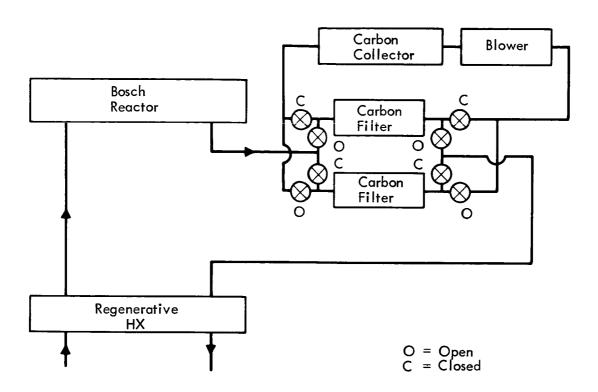
Figure B-5: CARBON REMOVAL — BOSCH
