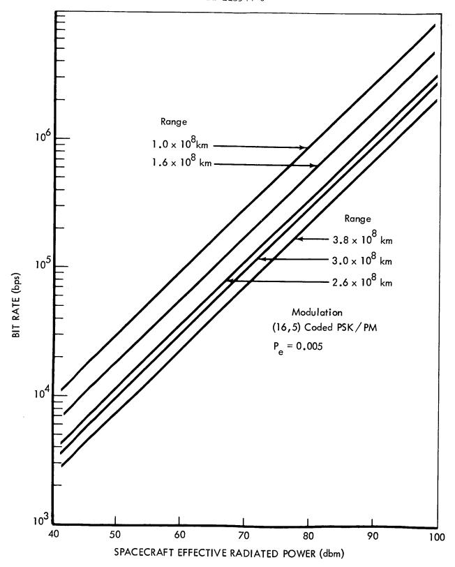
Figure 7.3-1: BIT RATE VERSUS RADIATED POWER (ERP)
