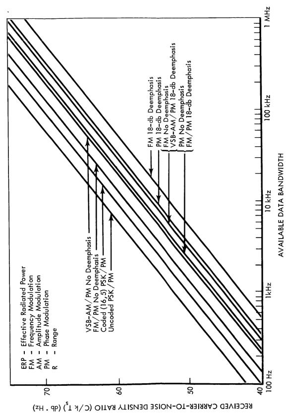
Figure C-3: COMPARISON OF THE BANDWIDTH CAPABILITIES OF ANALOG AND DIGITAL MODULATION TECHNIQUES
