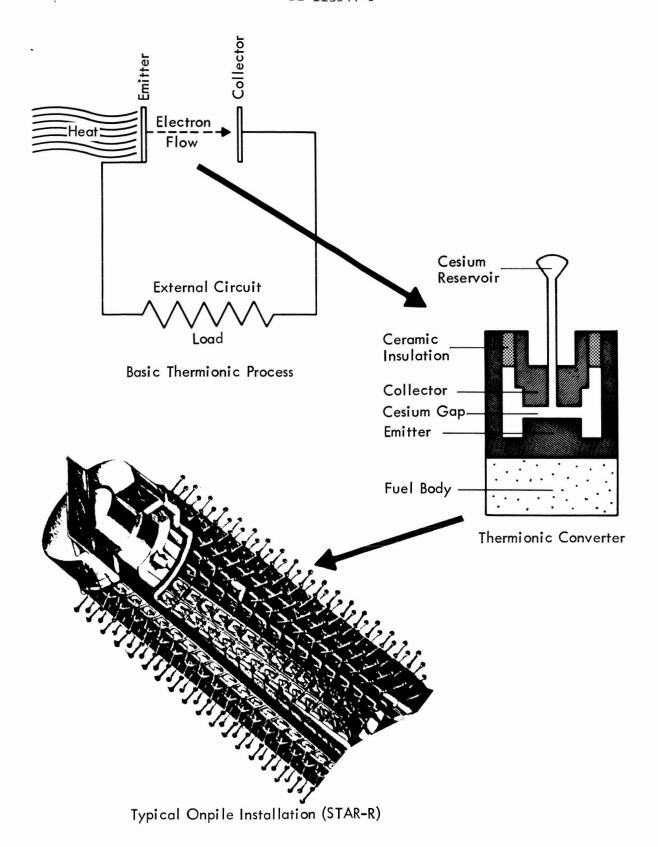
Figure A-12: THERMIONIC PROCESS AND EQUIPMENT
