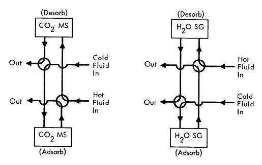
Figure B-1: CO<sub>2</sub> REMOVAL — MOLECULAR SIEVES
