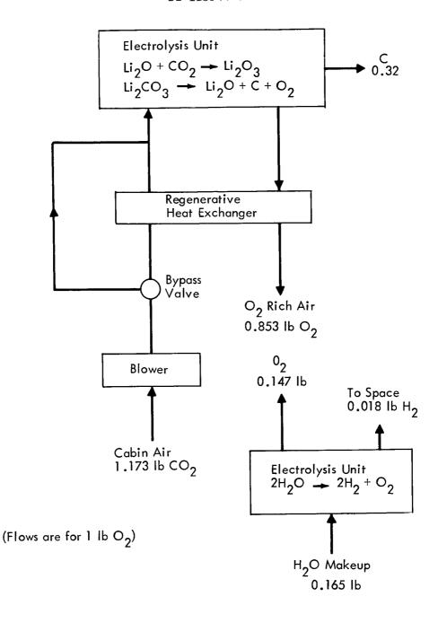
Figure B-8: CO<sub>2</sub> REMOVAL, O<sub>2</sub> RECOVERY — MOLTEN ELECTROLYTE
