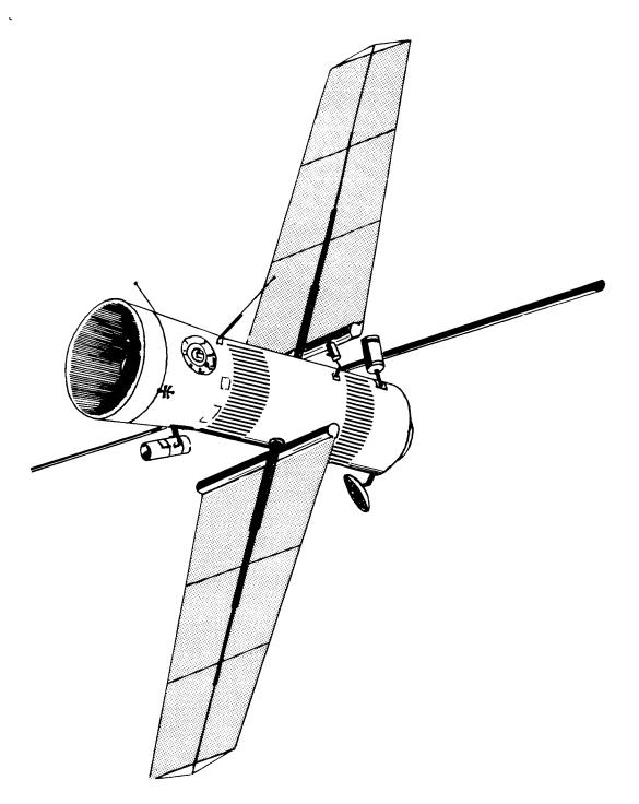
Figure A-2: TYPICAL ROLL OUT SOLAR ARRAYS
