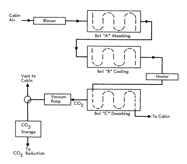
Figure B-3: CO<sub>2</sub> REMOVAL — SOLID AMINES
