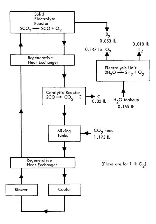
Figure B-7: O<sub>2</sub> RECOVERY — SOLID ELECTROLYTE
