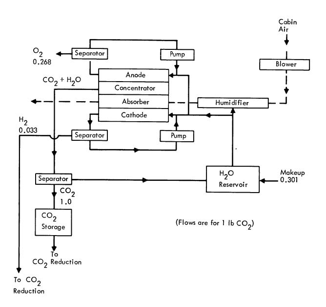
Figure B-2: CO<sub>2</sub> REMOVAL — ELECTRODIALYSIS
