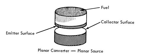
Figure A-13: TYPICAL CONVERTER-SOURCE GEOMETRIES FOR INPILE THERMIONIC CONVERSION
