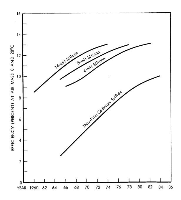
Figure A-3: ESTIMATED SOLAR CELL EFFICIENCY GROWTH TRENDS
