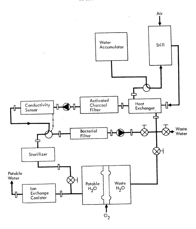
Figure D-3: VACUUM COMPRESSION DISTILLATION SYSTEM SCHEMATIC
