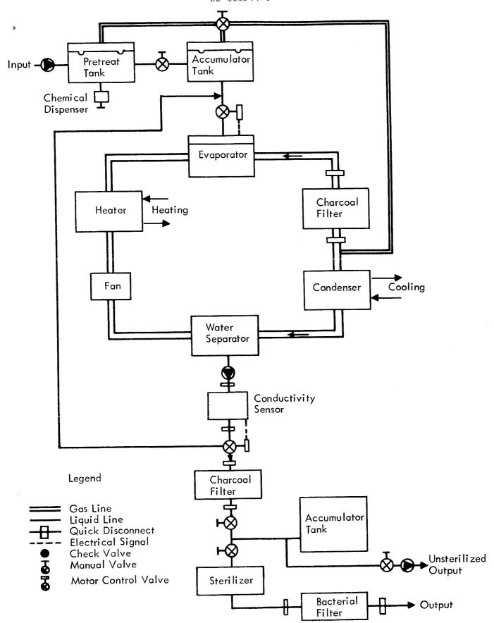
Figure D-2: AIR EVAPORATION WATER RECLAMATION
