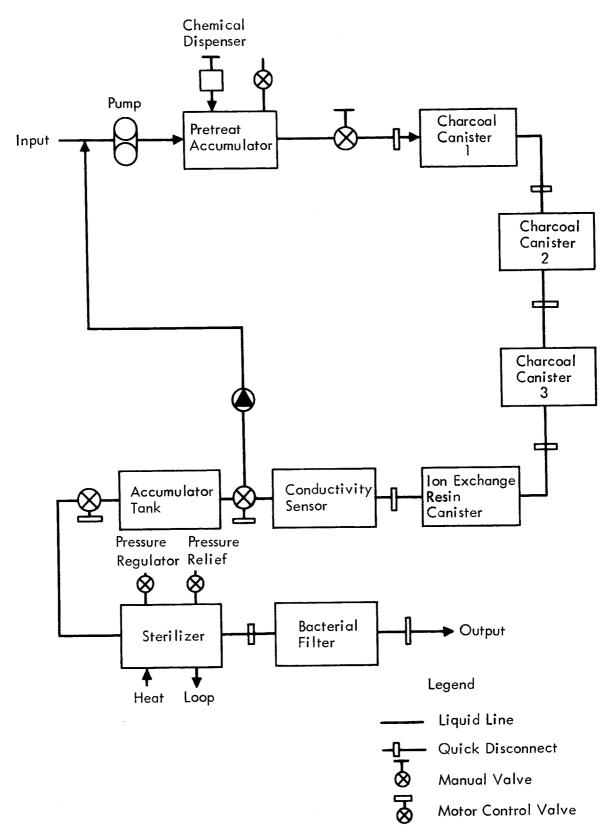
Figure D-1: MULTIFILTRATION WATER RECLAMATION
