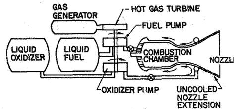
(a) Liquid-propellant rocket motor.
