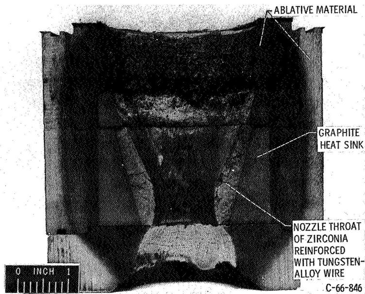
(c) Composite tungsten alloy-reinforced-zirconia nozzle after firing for 734 seconds.
