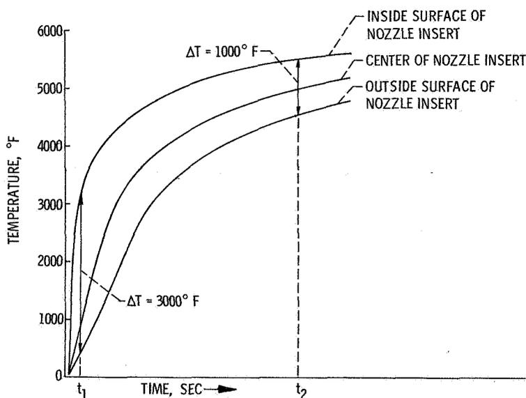
Figure 5-2. - Typical temperature distribution profiles in nozzle insert.
