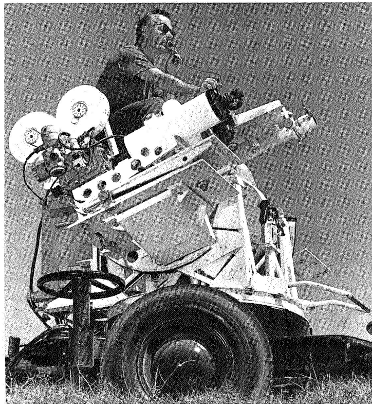
Figure 14-6. - Mobile optical trackers consisting of three to four cameras with lenses ranging in size from 20- to 120-inch focal length. These units are moved to suitable locations shown on Cape Kennedy map and operated by photographer seated on gimbal-mounted camera platform.
