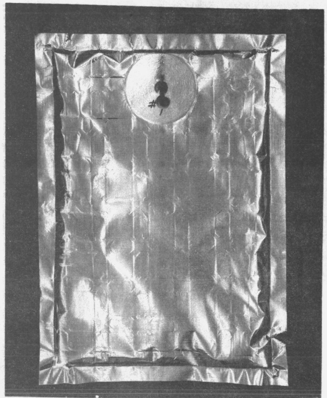
Figure 17 Recovered Panel Using Double Stripped Spacers
