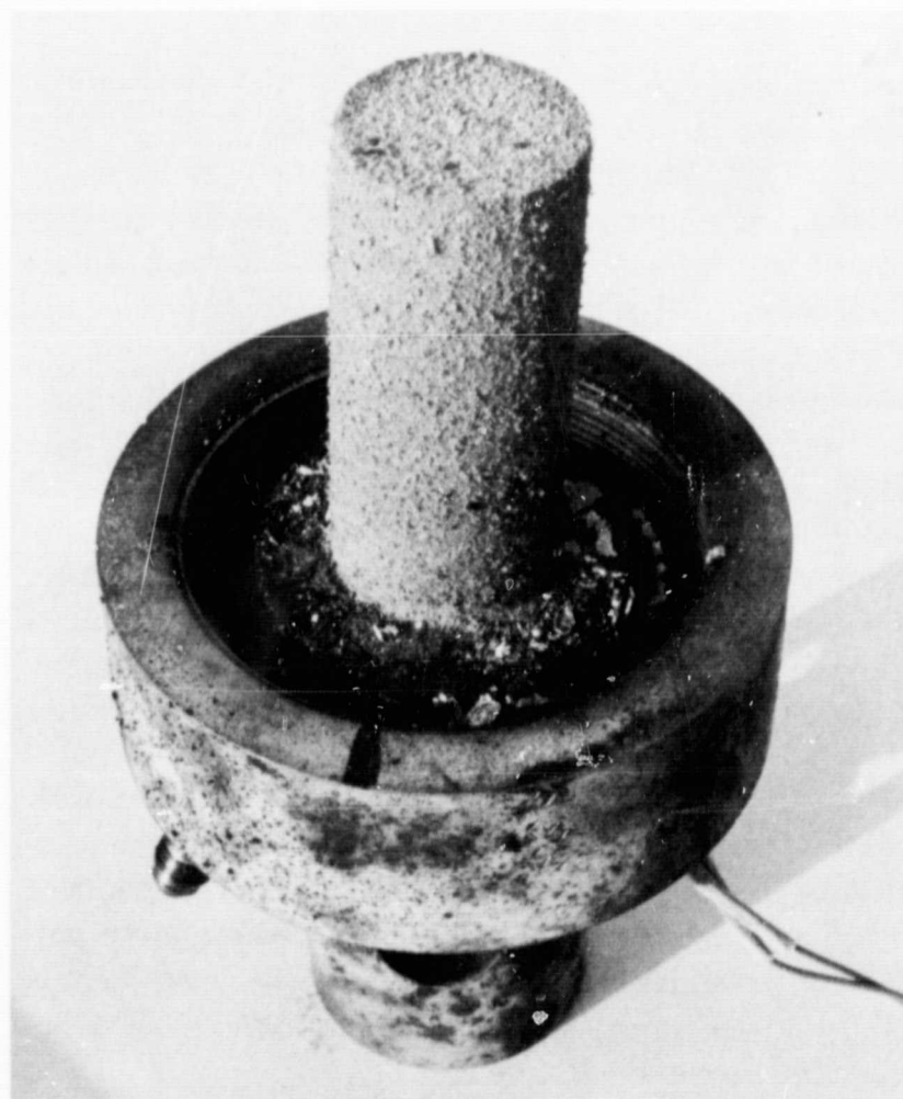
Fig. 15. Extinguished propellant grain, JPL 540 Mod 1 propellant
