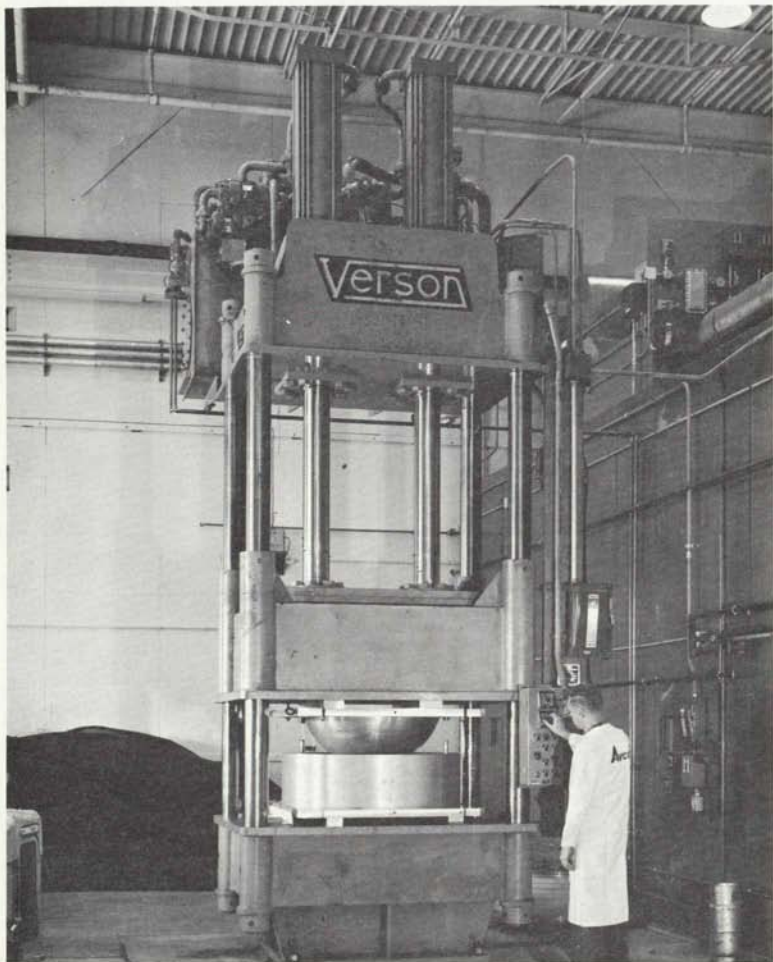
Photo No. 4-2. Avco Compression Molding Technique
