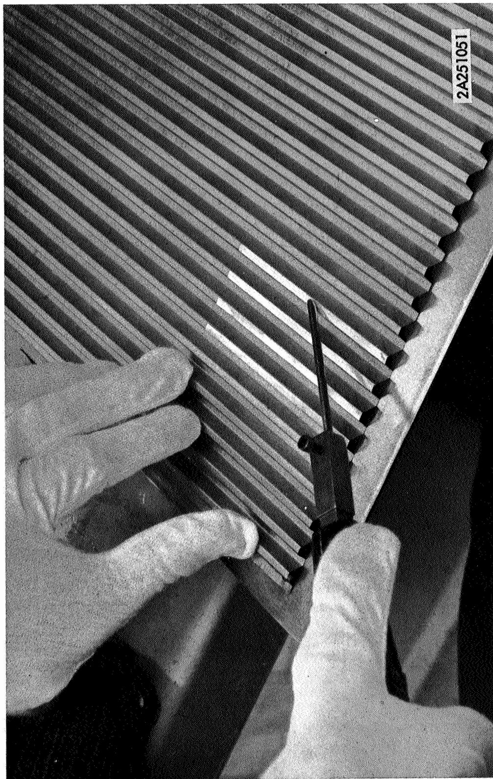
FIGURE 12 RESISTANCE SPOT TACKING OF BRAZE ALLOY TO BERYLLIUM CORE
