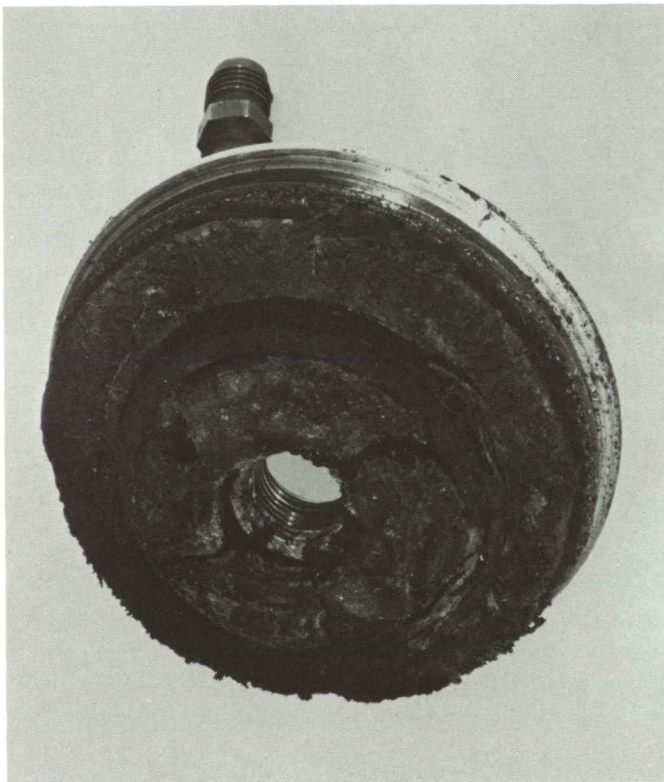
Fig. 33. ATS igniter closure, post-fire
