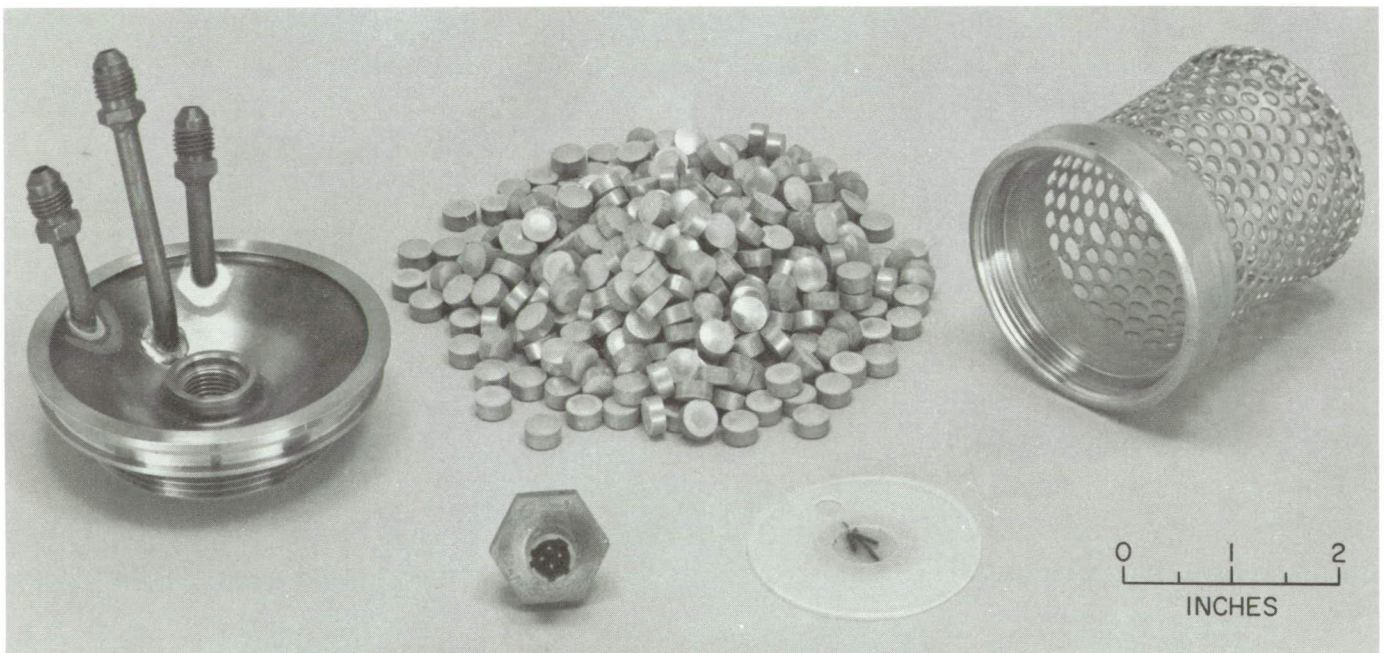
Fig. 9. Components of scaled-up Syncom igniter
