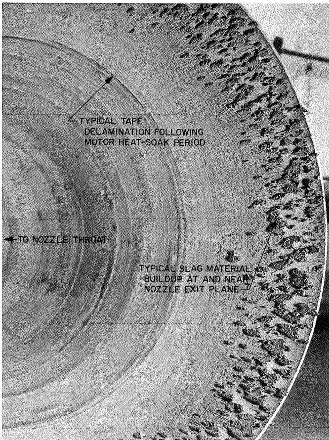
Fig. 20. Postfire condition of nozzle exit cone
