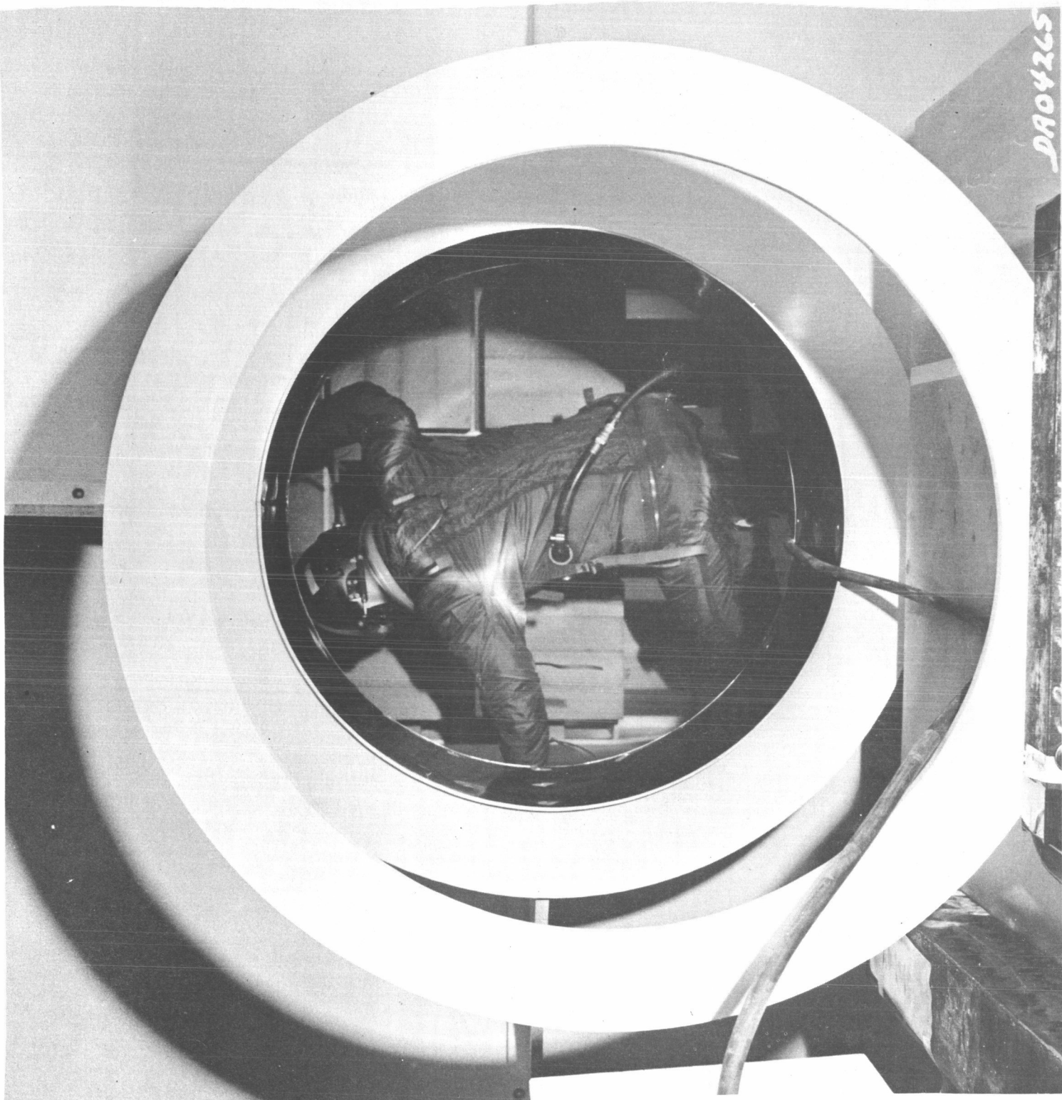
FIGURE 3.2.3-1, SUBJECT AT END AIRLOCK POSITION WITH SUIT UMBILICAL FROM CM (FULL SCALE MOCKUP)
