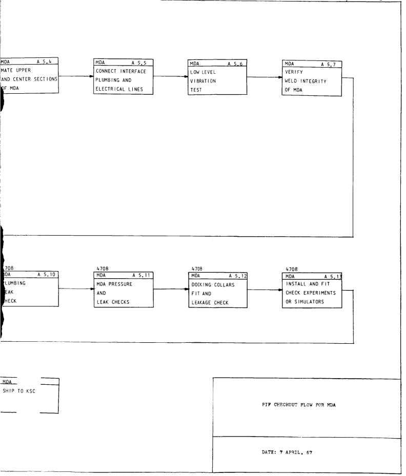
Figure 3. PIF Checkout Flow For MDA
