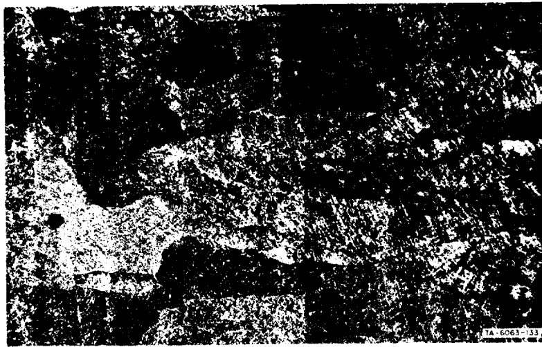
FIG. 18 PHOTOMICROGRAPH AT CENTER LINE OF LONGITUDINAL SECTION THROUGH GIRTH WELD; MAGNIFICATION, 20X (Etchant: 1 HF, 4 HNO 3 , 95 H 2 O, swab 10 seconds)
