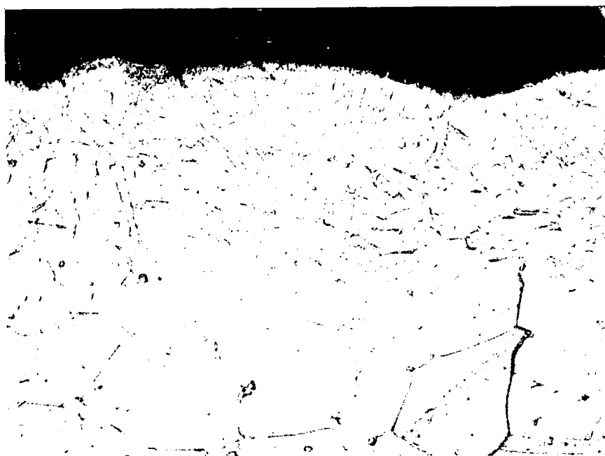
FIGURE 17. Pure Titanium, 0.005" Thick, 900X, One Electrical Discharge. Note Region of Overheating and Fusion Next to Surface. The Immediate Surface Layer had been Melted.
