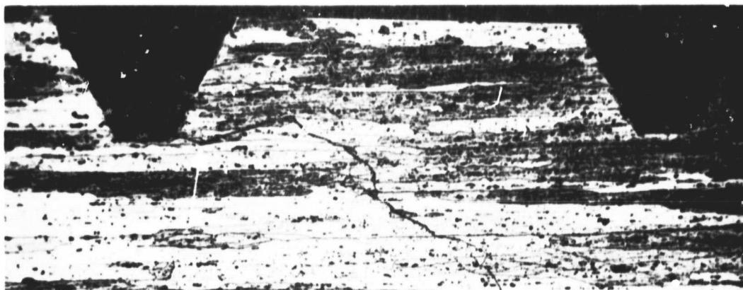
B FAILURE OCCURRING AT ROOT OF THREAD
