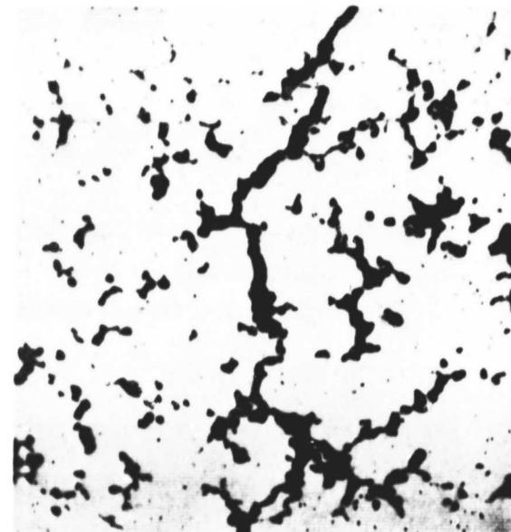
C MICROGRAPH OF CRACKED AREA
