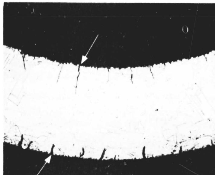
D MICROGRAPH OF CONVOLUTION WITH PARTIAL
