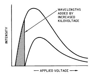
Figure 2-10. Effect of Increasing Voltage on the Quality and Intensity of an X-Ray Beam
