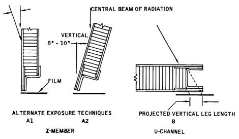
Figure 6-42. Vertical Tie Exposure
