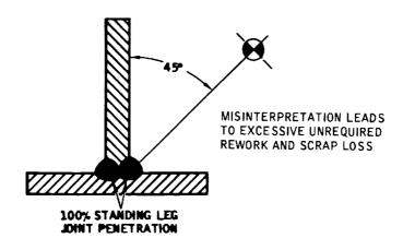
Figure 6-23. Correct Angle for T-Joint (100% Standing Leg Penetration)
