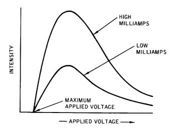
Figure 2-11. Effect of a Change in Tube Current on an X-Ray Beam
