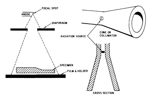
Figure 6-1. Diaphragm, Collimator and Cone
