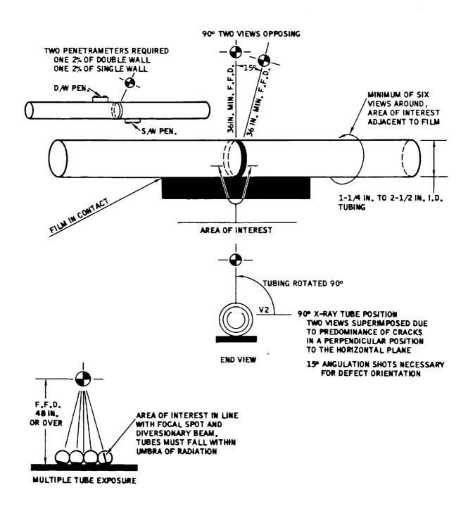
Figure 6-29. Double Wall Application with Tube Size Over 1 1/4 Inch Inside Diameter
