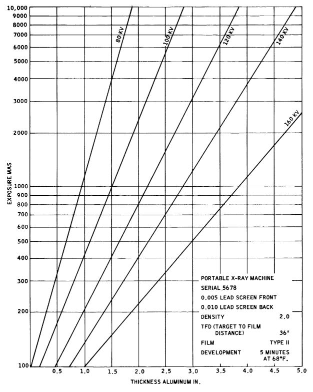
Figure 6-11. X-ray Exposure Chart (Portable Equipment)
