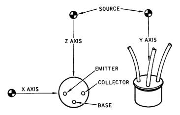
Figure 6-45. Suggested Views of Transistor
