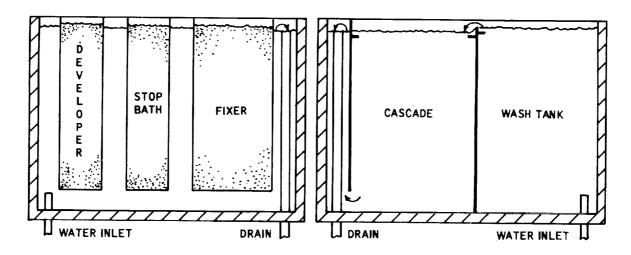
Figure 4-6. Typical Tank Processing Unit
