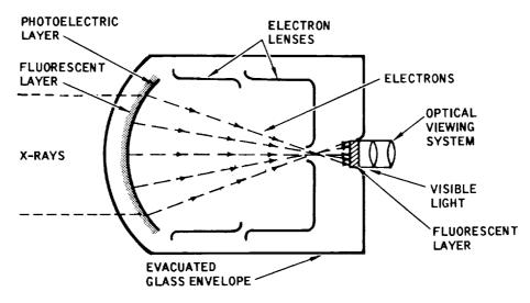
Figure 6-48. Schematic of an Image Amplifier
