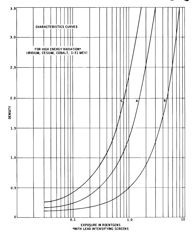
Figure 6-15. Film Characteristic Curves (Types A, B and C)
