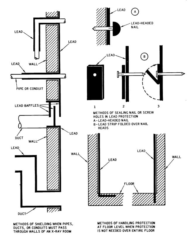
Figure 5-2. Radiation Protection Constructions
