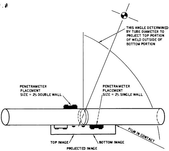
Figure 6-30. Double Wall Application with Tube Size Less Than 1-1/4 Inch Inside Diameter
