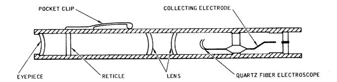
Figure 5-6. Pocket Dosimeter (Typical)
