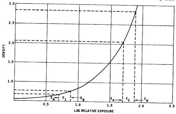
Figure 4-3. Film Characteristic Curve
