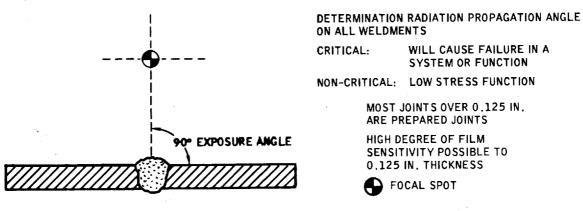
Figure 6-19. Common Buttweld
