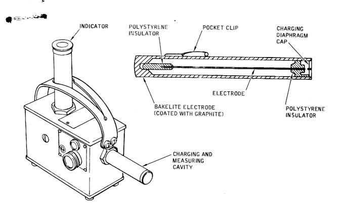
Figure 5-7. Pocket Chamber and Charger (Typical)
