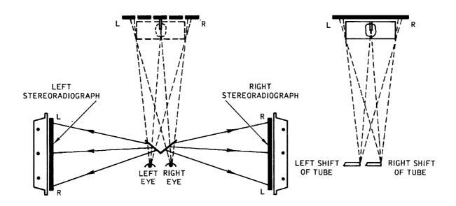
Figure 6-51. Stereoscopic Radiography
