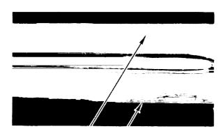
A FRACTURED SPECIMEN SHOWING UNFUSED POROSITY
