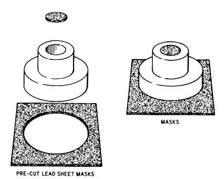
Figure 6-3. Lead Masking Technique
