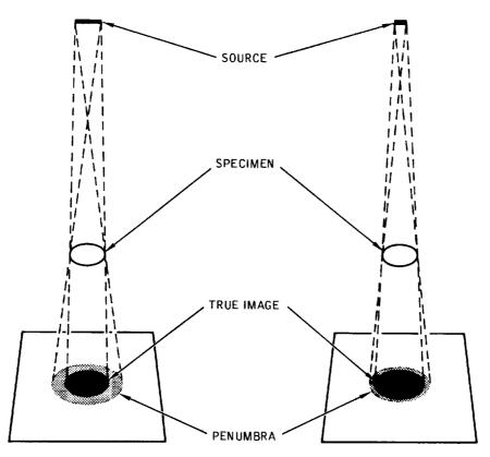
Figure 2-4. Effect of Source Size on Image Sharpness
