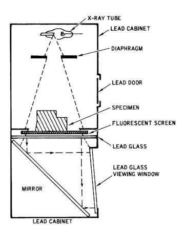
Figure 6-47. Schematic Diagram of a Fluoroscope
