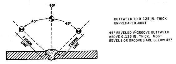
Figure 6-20. V-Groove Buttweld
