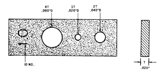
Figure 6-5. Standard Penetrameter for 1" Material
