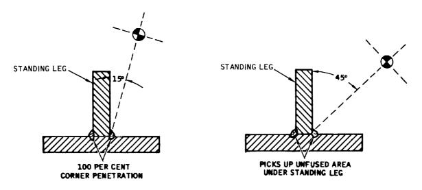
Figure 6-21. Correct Angle for T-Joint Figure 6-22. Incorrect Angle for T-Joint (100% Corner Penetration)
