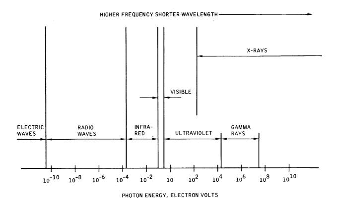
Figure 2-6. The Electromagnetic Spectrum
