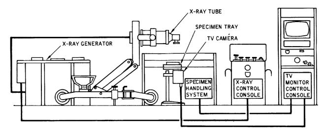
Figure 6-49. Typical Vidicon X-ray System
