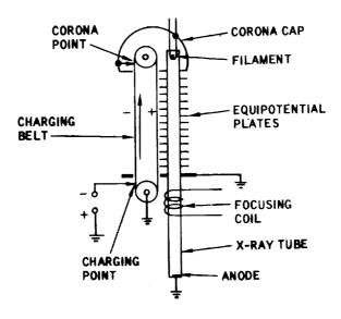
Figure 3-7. Diagram of Electrostatic Generator
