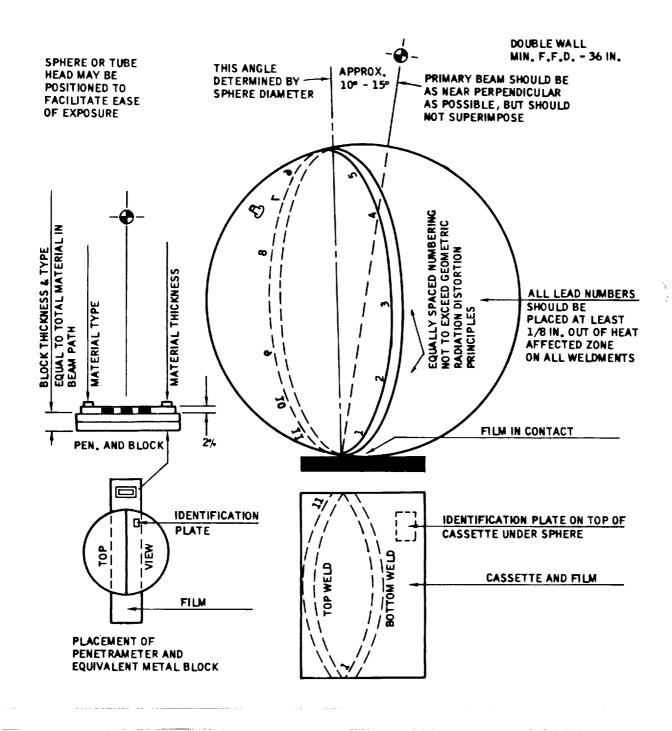
Figure 6-31. Sphere Weldment Application
