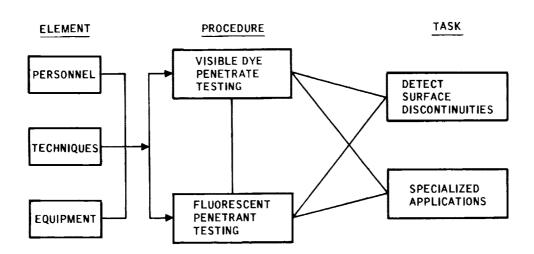
Figure 7-1. Liquid Penetrant Test
