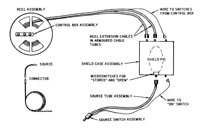
Figure 3-10. Diagram of Typical Isotope Camera
