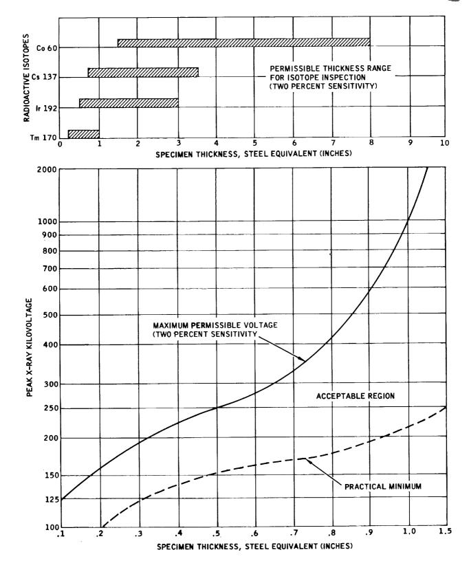
Figure 6-17. Energy vs. Thickness Ranges
