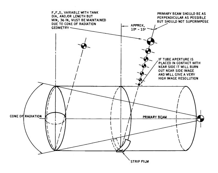
Figure 6-32. Closed Tank Application
