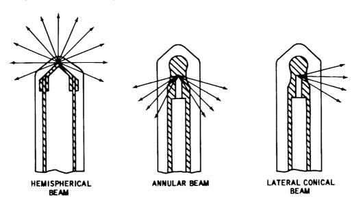
Figure 3-4. X-Ray Beam Configuration
