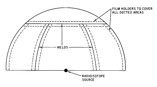
Figure 6-34. Hemispherical Section
