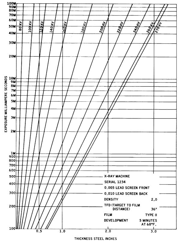
Figure 6-12. X-ray Exposure Chart (Permanently Installed Equipment)
