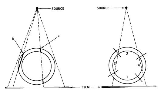
Figure 6-37. Large Pipe Welds
