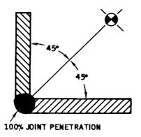
Figure 6-26. Correct Angle for Corner Joint and Correct Detail Placement (100% Penetration)
