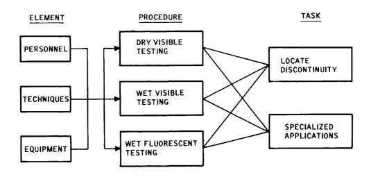
Figure 7-2. Magnetic Particle Test
