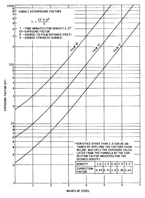
Figure 6-8. Gamma Ray Exposure Chart
