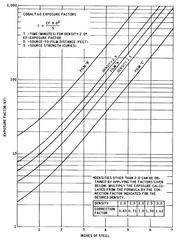
Figure 6-9. Gamma Ray Exposure Chart (Modified)
