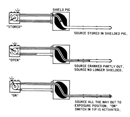
Figure 3-11. Operation of Typical Isotope Camera
