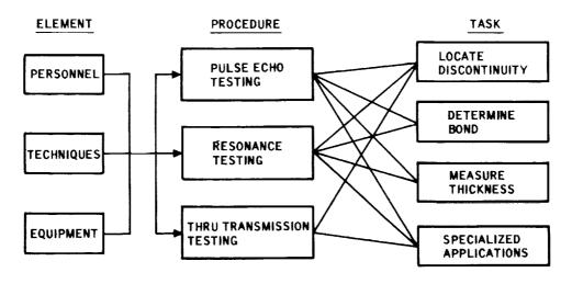
Figure 7-3. Ultrasonic Test
