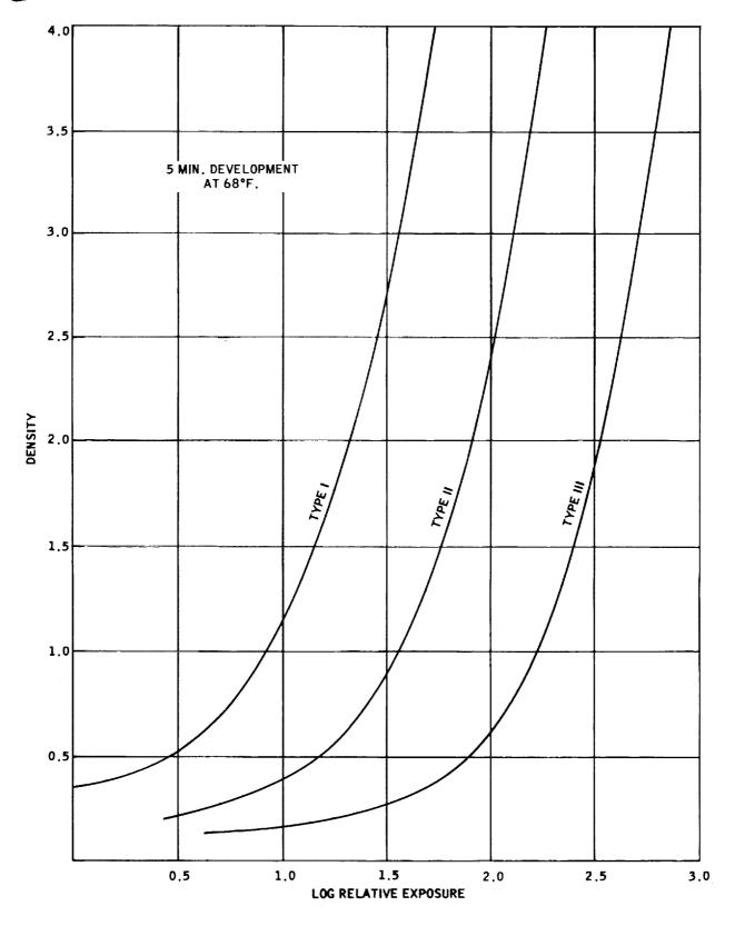
Figure 6-14. Film Characteristic Curves (Types I, II and III)
