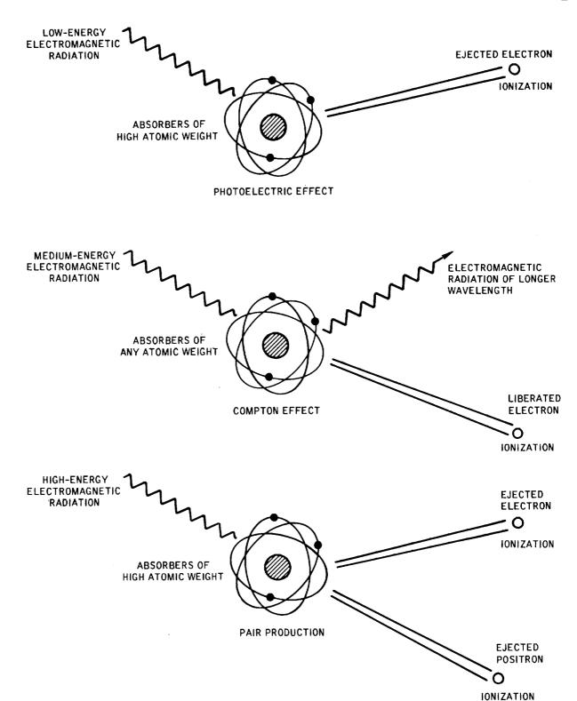
Figure 2-12. Ionization by Electromagnetic Radiation
