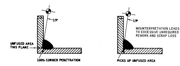
Figure 6-24. Correct Angle for Corner Figure 6-25. Correct Angle for Corner Joint and Correct Detail Placement Joint but Incorrect Detail Placement
