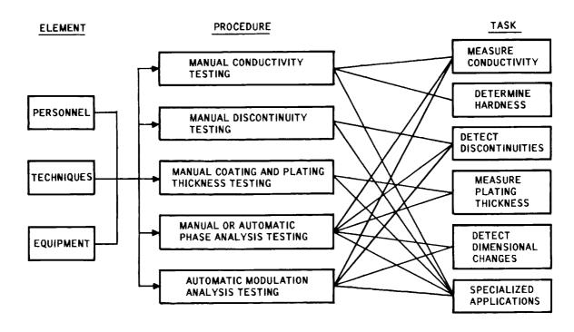
Figure 7-4. Eddy Current Test
