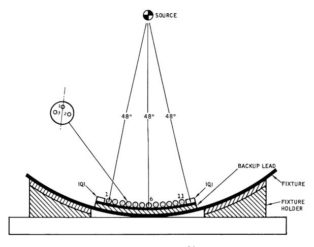
Figure 6-44. Semiconductor Holding Fixture
