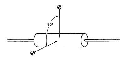
Figure 6-46. Suggested Views of Diode, Resistor, and Capacitor
