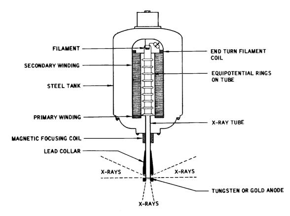
Figure 3-6. Resonant Transformer X-Ray Equipment
