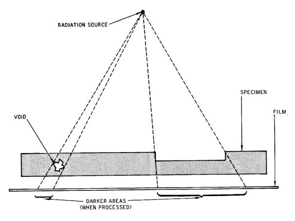
Figure 2-1. Basic Radiographic Process
