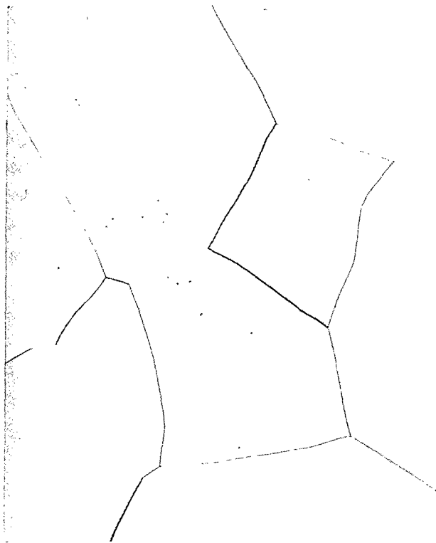
(a) Buttonhead; average grain diameter, \approx 300 micrometers.
