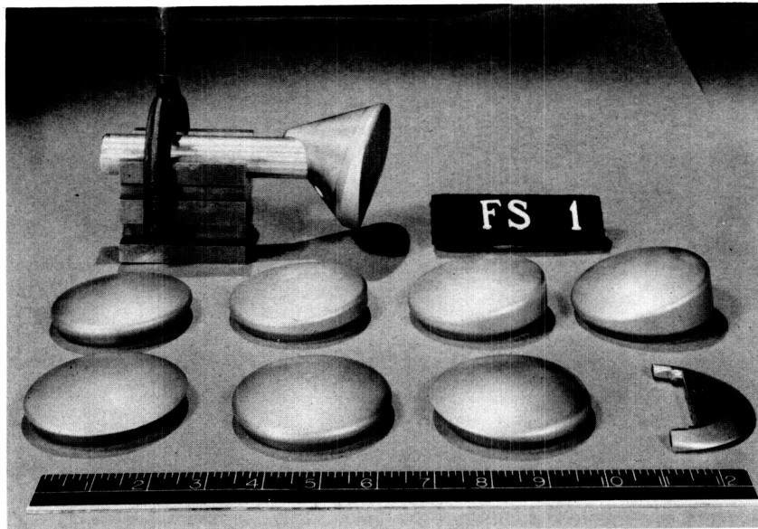
(c) Photograph of 0.02-scale model, showing various modifications tested for lift-to-drag ratio improvement.
