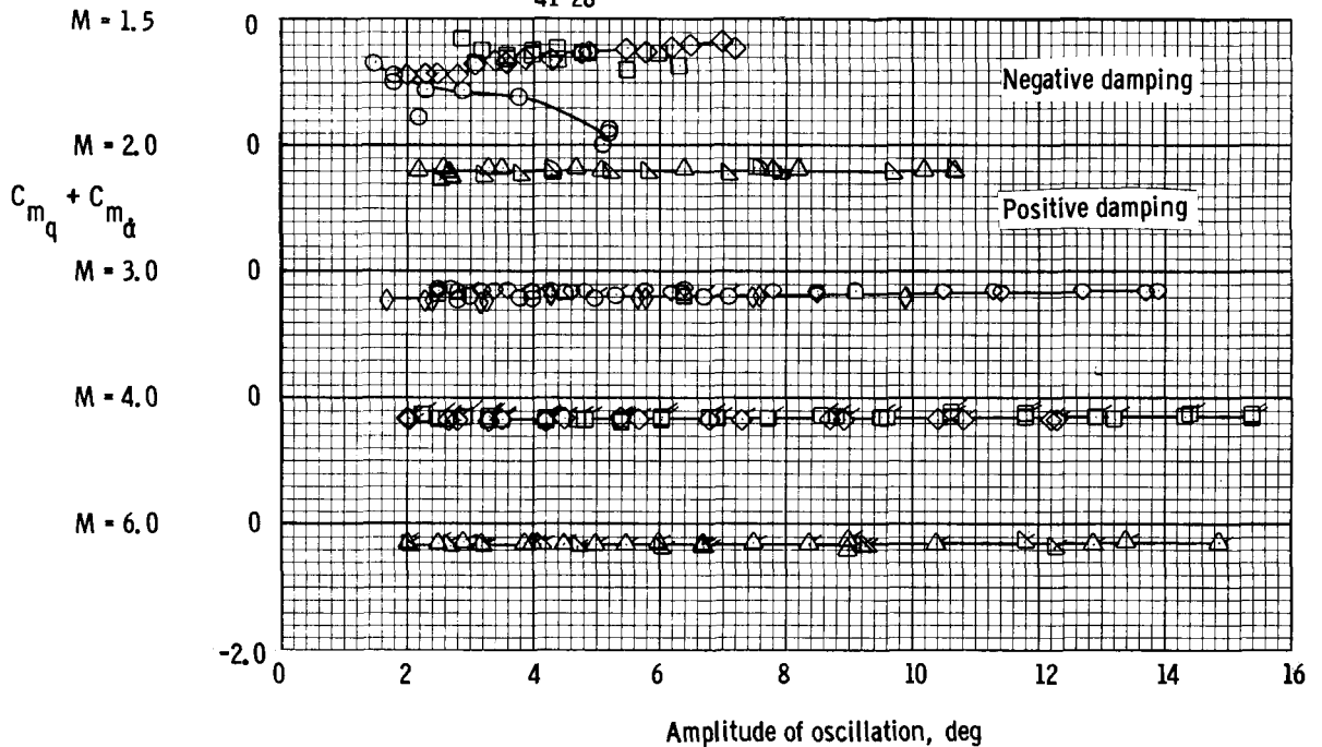
Figure 27. - Longitudinal oscillatory stability derivatives of the Apollo command module with strakes obtained at AEDC-A facility at M = 1.5 to M = 6.0 .
