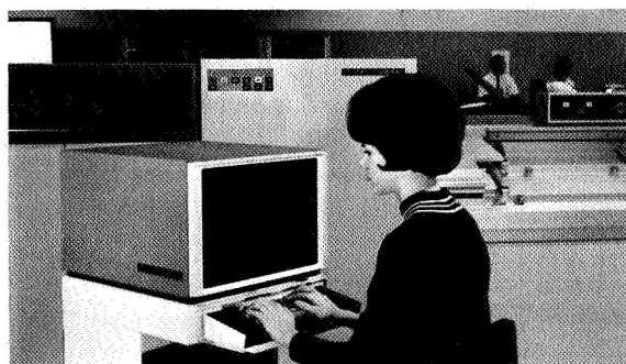
FIGURE 38.—Airline reservation system display console. Agent set for Burroughs airline reservation system built for TWA. This newer airline reservation system uses CRT displays for rapid display of information to the agent in response to his requests for reservation status of given flights.
