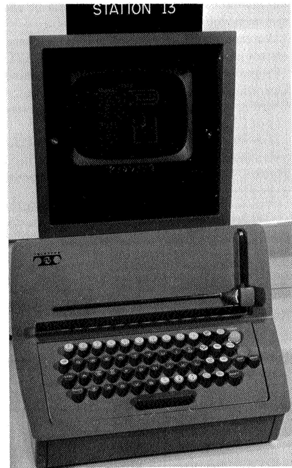
FIGURE 37.—A PLATO student terminal device. The student sees information on a TV-screen (which is an ordinary 525-line TV monitor), and he enters information by means of a teletypewriter keyboard, similar to an ordinary typewriter.
