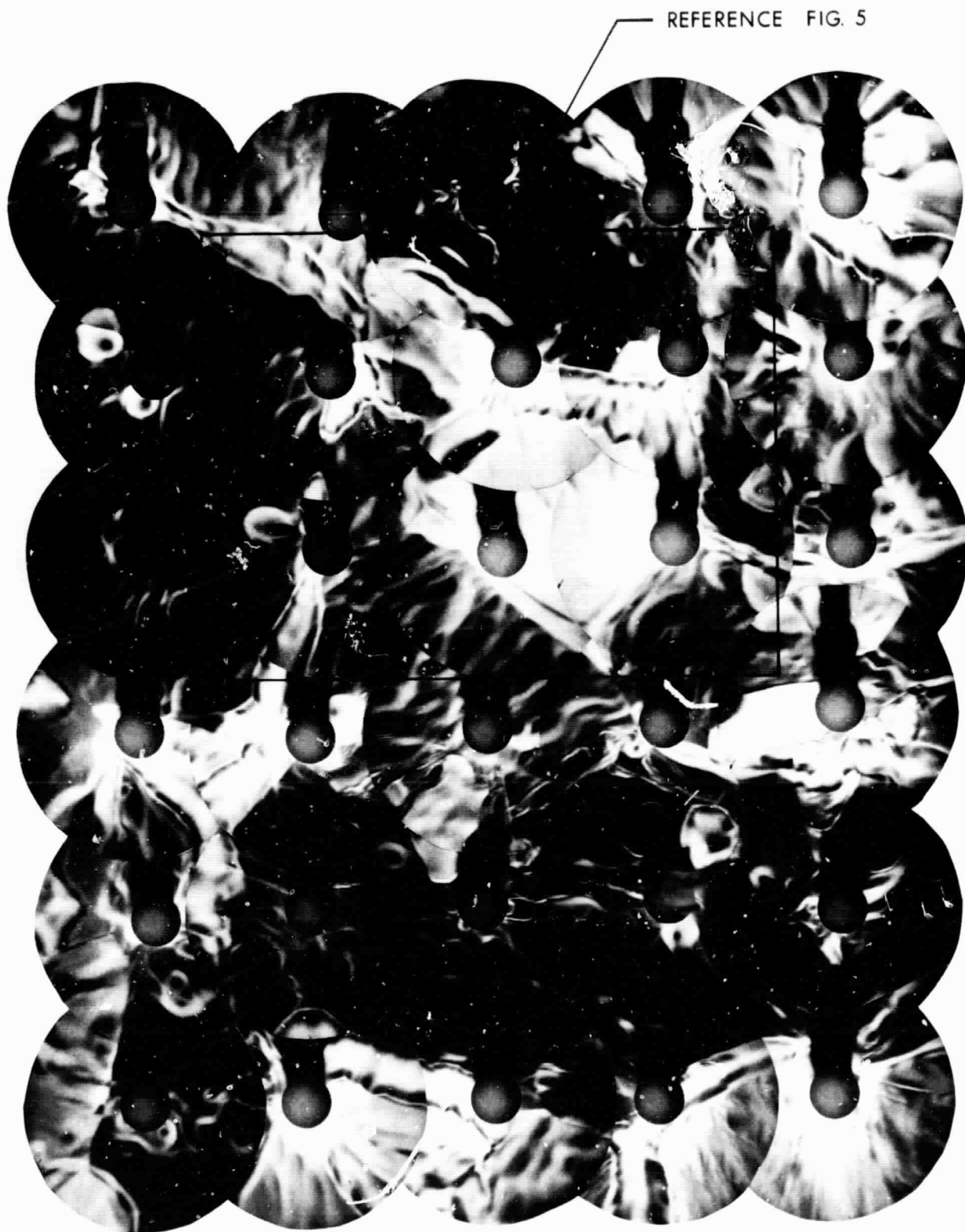
Figure 28. Composite After Electro-Etch of Mapped Area (12 mil square) ( \times 200 )
