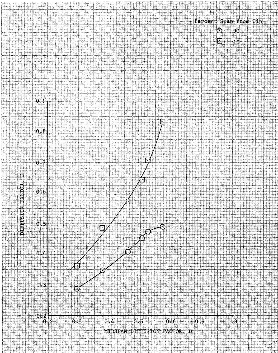
Figure 23. Hub and Tip Diffusion Factor as a Function of Midspan Diffusion Factor - Flow Generation Rotor (Slotted Stator 3 Test), Design N/\sqrt{\theta}
