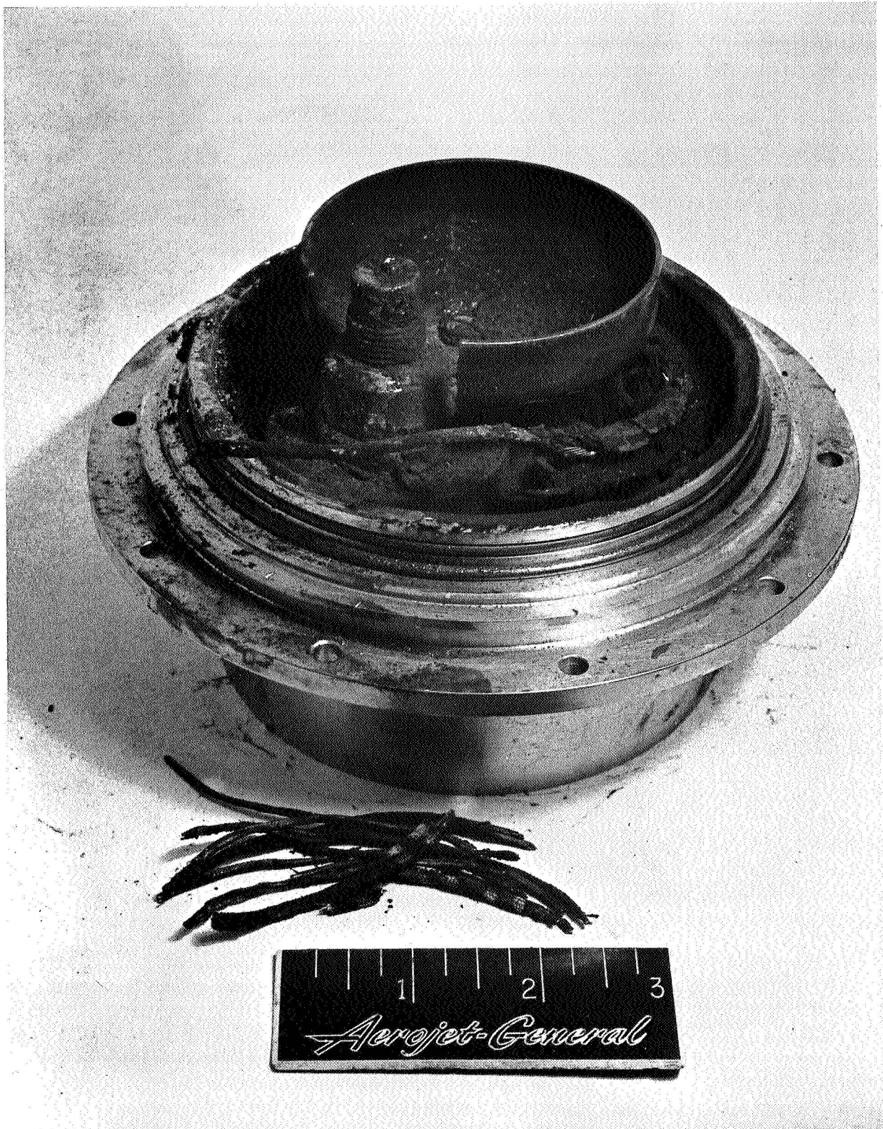
Motor From Mercury PMA, Showing Damage Due to Mercury Contact After 938 Hours of Operation (View 1)
