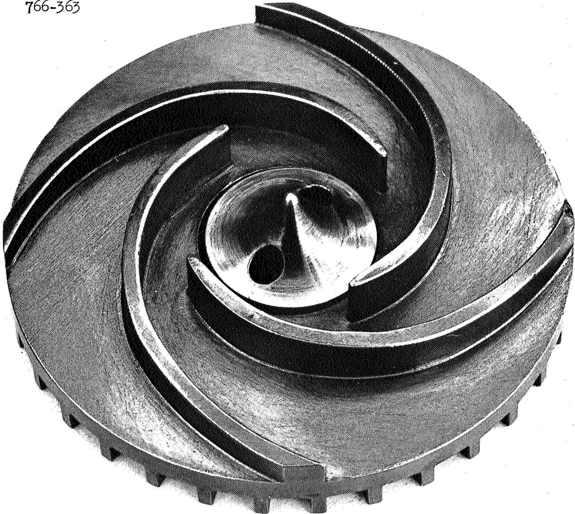
Impeller and Bolt From Mercury PMA (P/N 093347-5, S/N A-1) After 1099 Hours of Operation in PCS-1
