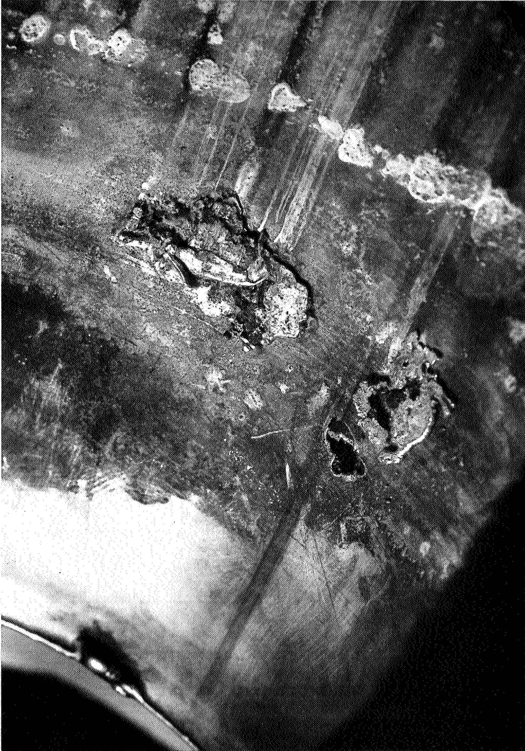
Inside Bore of Stator Can From NaK PMA Unit 4/1 (P/N 093200-13C, S/N A-4), Showing Arc Holes and Copper Splatter at Areas 3 and 4
