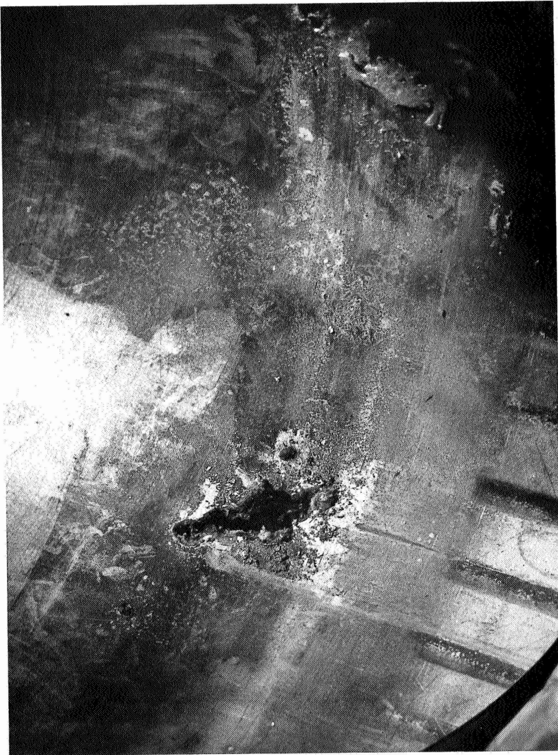
Inside Bore of Stator Can From NaK PMA Unit 4/1(P/N 093200-13C, S/N A-4), Showing Arc Holes at Area 5
