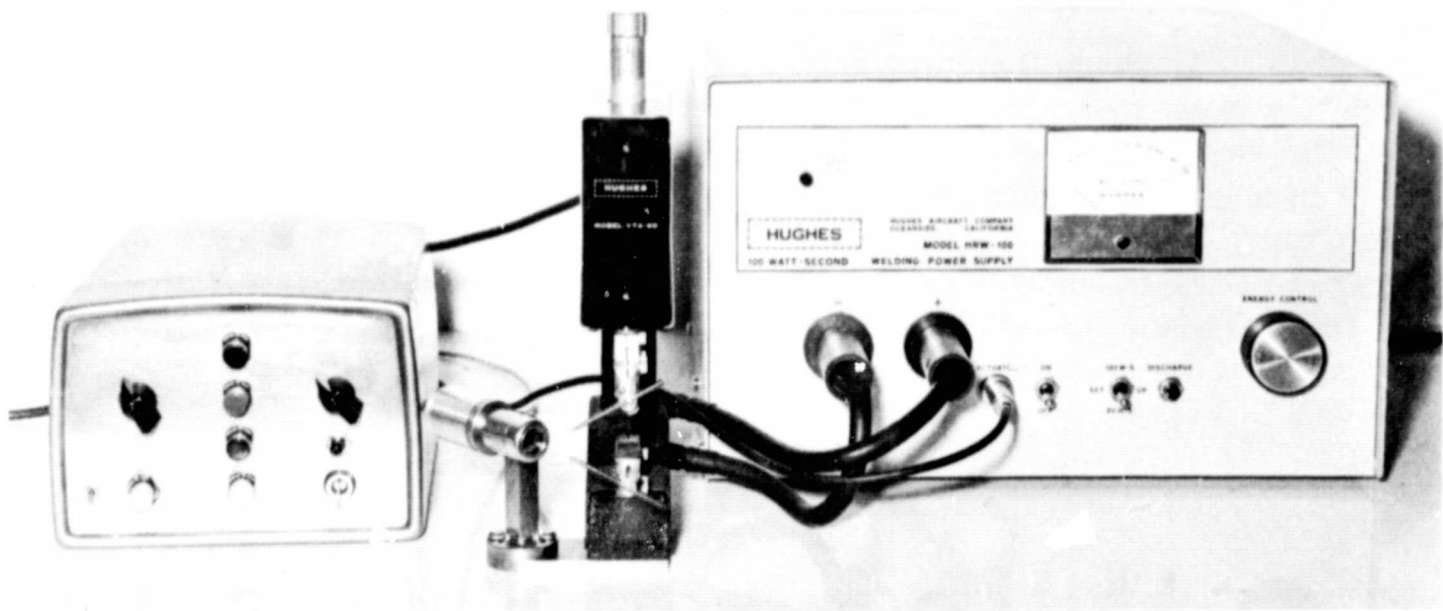
Figure 2. Infrared Radiation Weld Evaluator Engineering Prototype System
