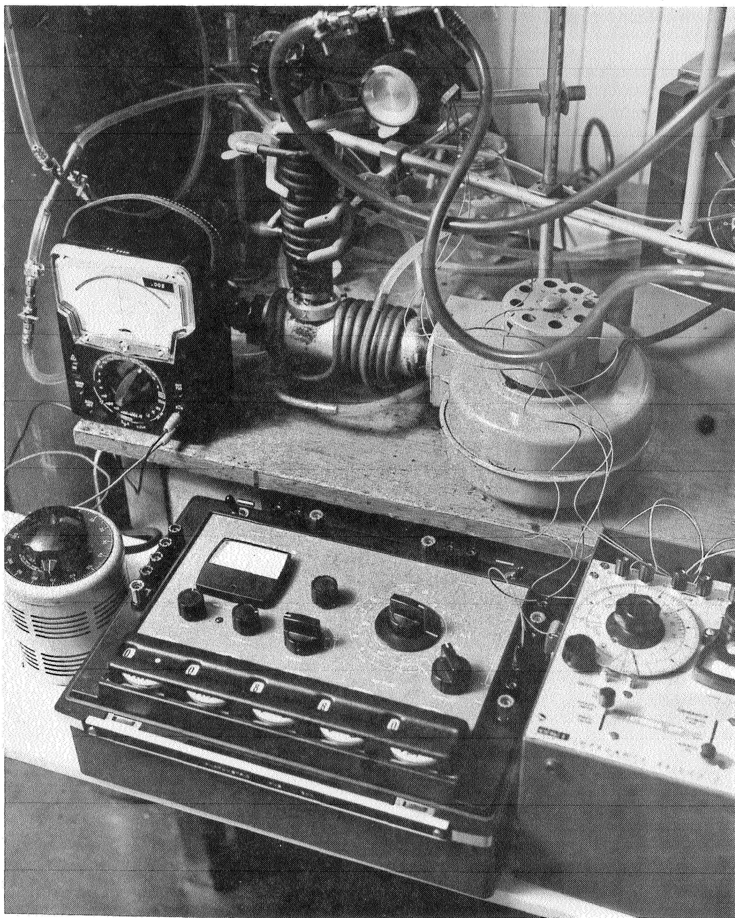
Figure FR-21. Spectrophotometric Studies of Whole Blood, Backscatter Mode: Detail of pump-oxygenator flowthrough cuvette apparatus showing cooled lamp housing and equipment for measuring the intensity of light backscattered from whole blood.
