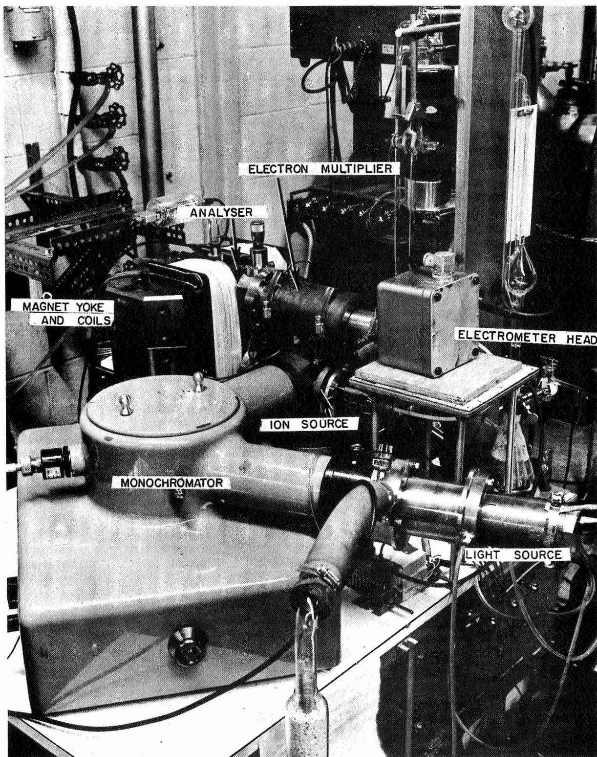
Figure 4. Photograph of photoionization-mass spectrometer setup.
