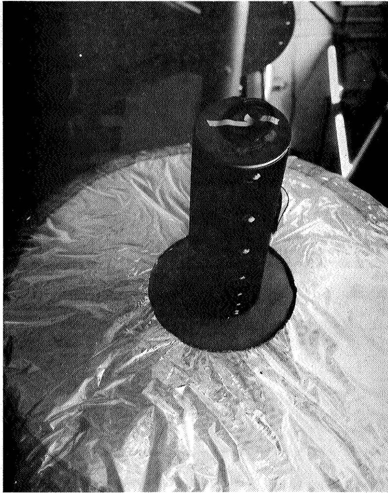
FIGURE 27 UNINSULATED "A" CAP PIPE PENETRATION ATTACHED TO TANK CALORIMETER
