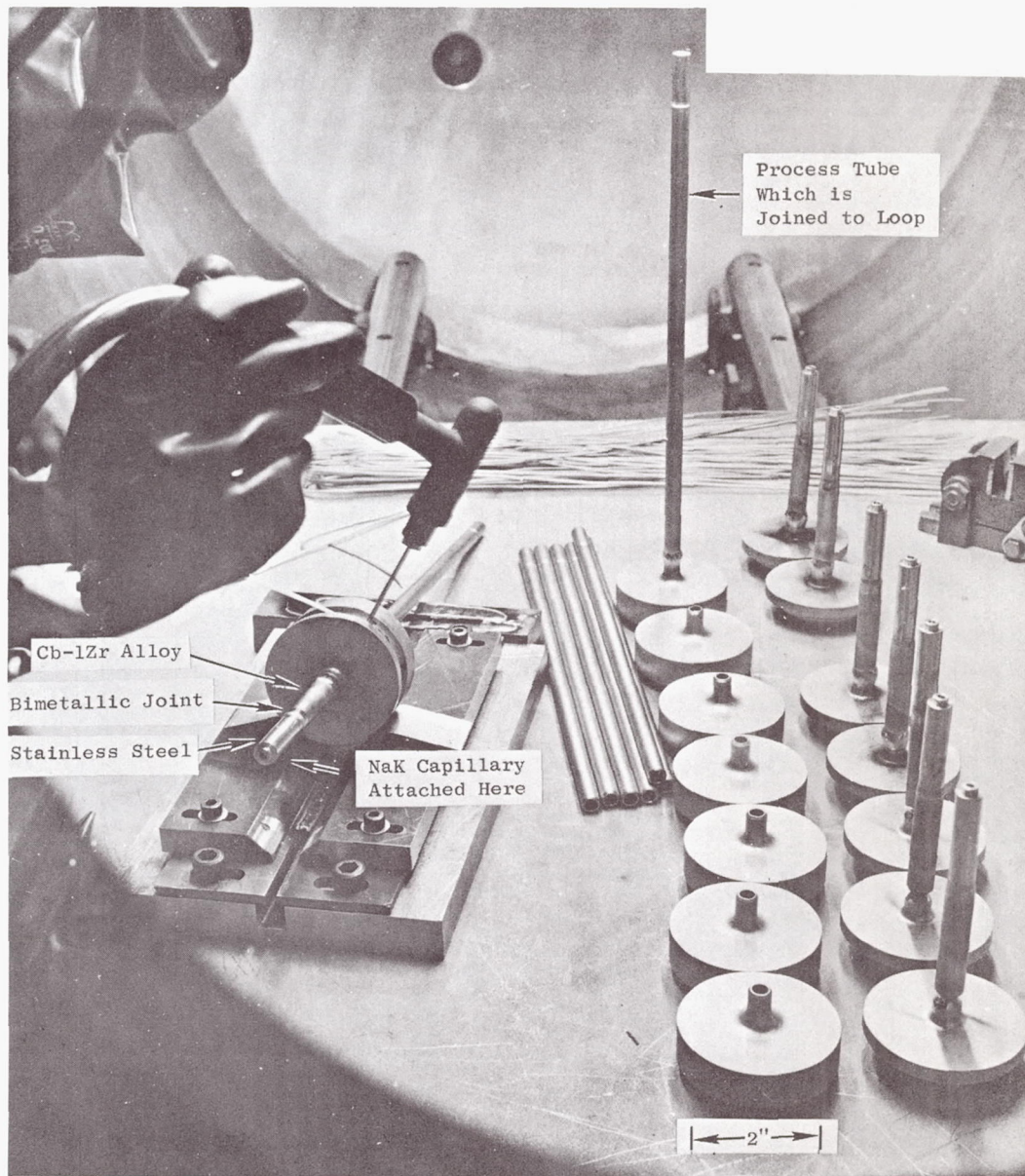
Figure 23. Photograph Taken Through the View Port of the Welding Chamber During the TIG Welding of the Slack Diaphragm Pressure Transducer Housings. (Orig. C64013149)
