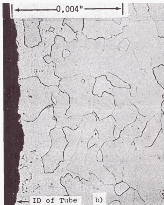
Figure 72 Microstructure of a Typical Cross Section of the Sodium - Cb-1Zr Pump Tubing (0.375" OD x 0.065" Wall) Before Test. Etchant: 60 ml Glycerine - 20 ml Hf - 20 ml \text{HNO}_3
