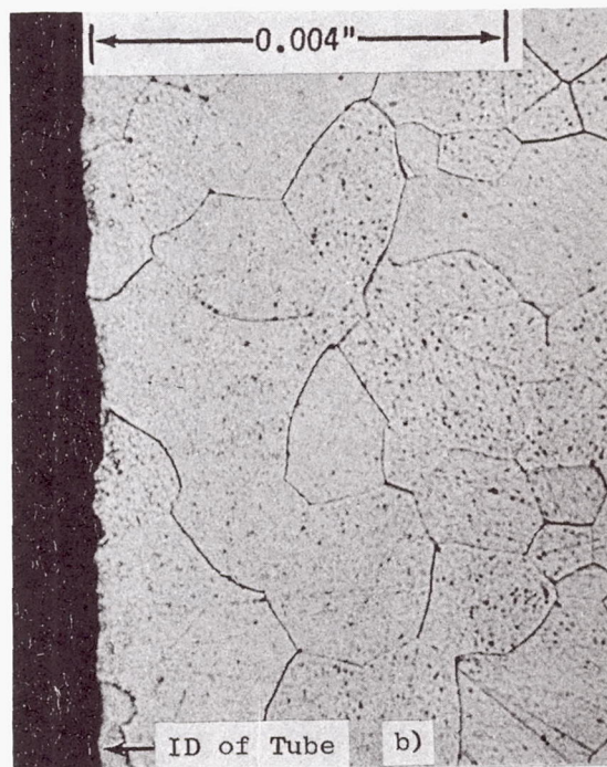
Figure 73 Microstructure of a Cross Section of the Cb-1Zr Tube From the Region Six Inches Below Lower Heater Electrode, Region C in Figure 70, 1965°F.
