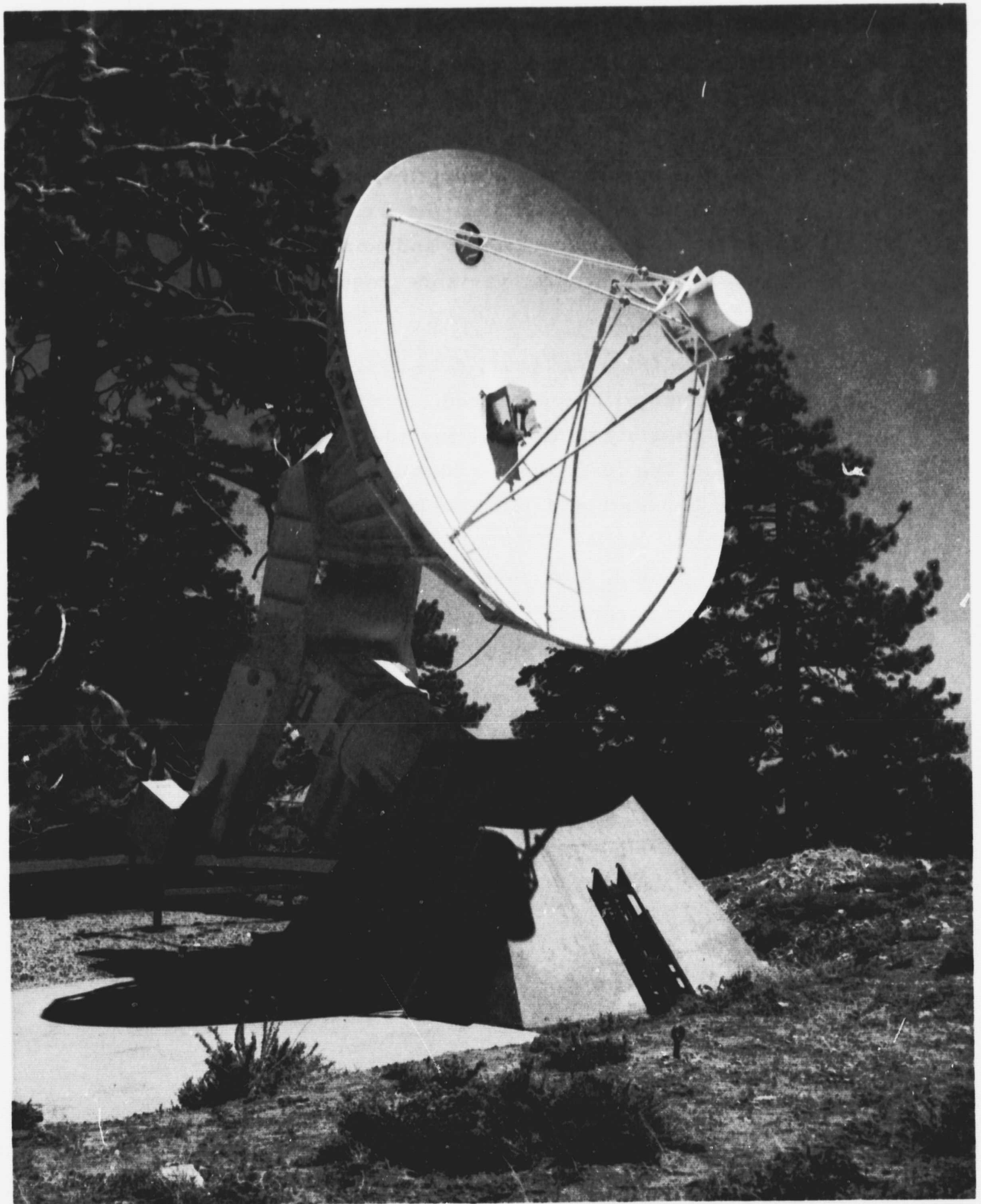
Figure 1. 18-ft Antenna After Rework
